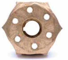
WORN DRIVE PLUG Accelerated wear due to lack of drain holes in a look-alike brush
