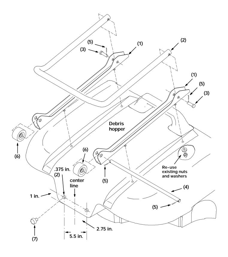
FIG. 1 - Dump Assist Kit Assembly
