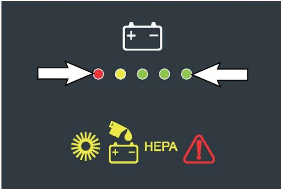
When the batteries are fully charged, all five indicators are illuminated. Recharge the batteries when there is only one indicator illuminated. Do not allow the batteries to discharge below 20% (last indicator).
