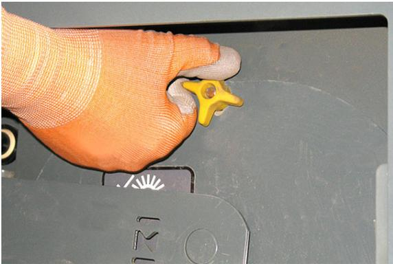
4. Remove the idler arm assembly from the main brush assembly.
