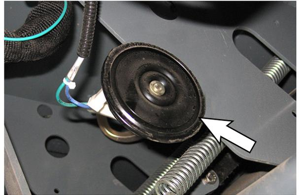
7. Inspect connections at pins/terminals for signs of corrosion/damage.
