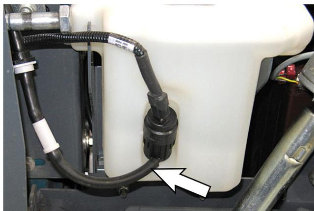
9. Remove the battery water delivery assembly from the machine.
