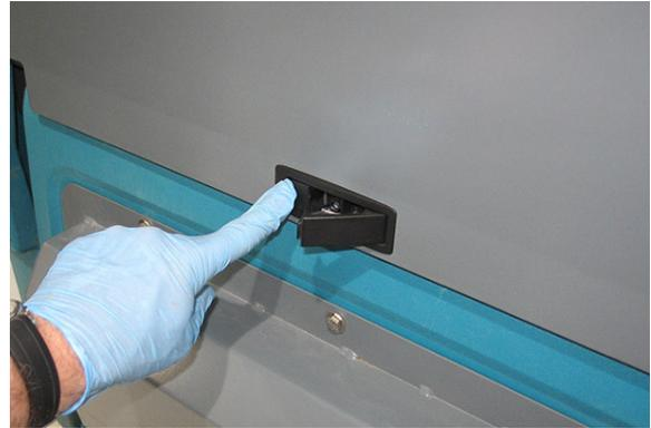
2. Lift the vacuum wand housing cover open and use the prop rod to secure the cover open.
