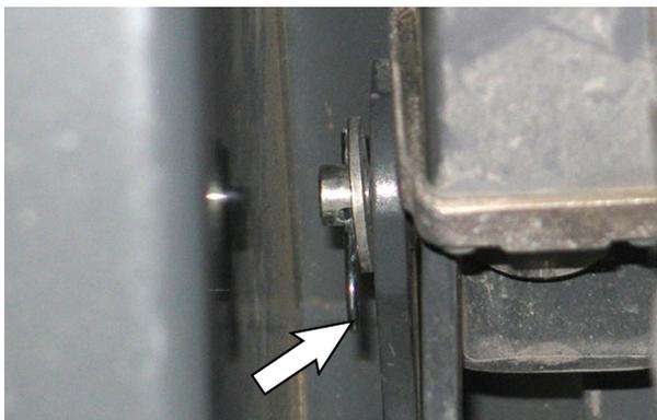
7. Secure the hopper into the rolled in position so hopper does not roll when clevis pins are removed from the rollout actuator and the left hopper mounting plate and follower plate.
