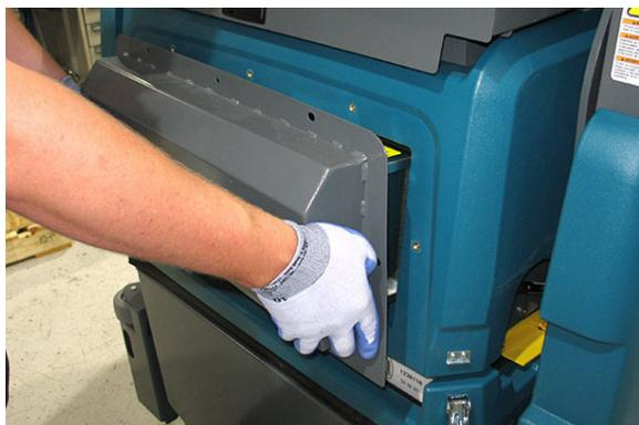
3. Remove the hardware securing the HEPA filter to the HEPA tray and remove the HEPA filter from the tray.
