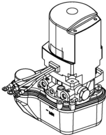
3. Use fuse-protected jumper leads to apply battery voltage to the pump motor. Connect battery positive (+) to green wire and battery negative (-) black wire. The motor should engage hydraulic cylinder to lower.
