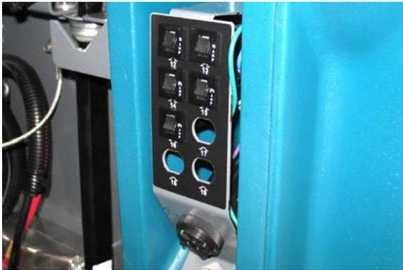
If the overload that caused the circuit breaker to trip is still present, the circuit breaker will continue to stop current flow until the problem is corrected.
