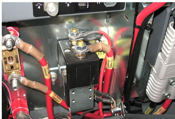
7. Confirm connections at B- and B+ main sweep circuit board. Secure/repair connections.
