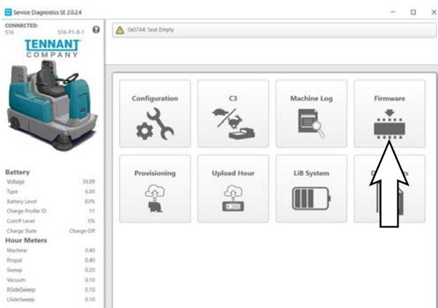
Allow the firmware update package to update the machine operating system. Various update status indicators appear on the screen while the firmware updates are occurring. Watch the visual status indicators on the screen for the update status.
