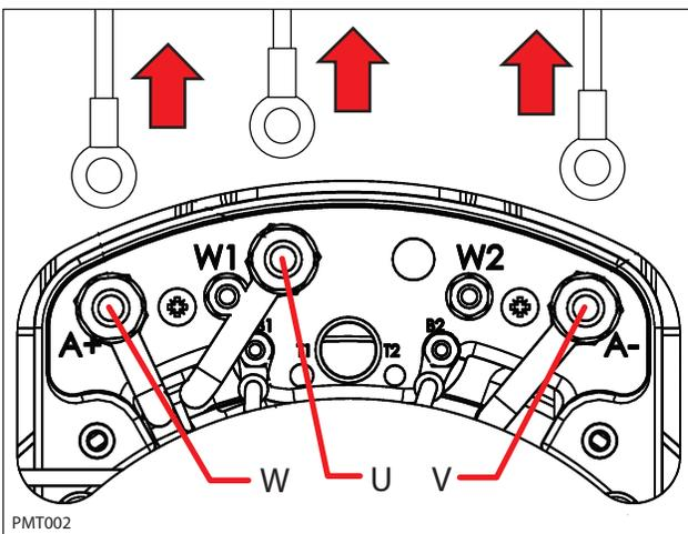
4. Disconnect U, V, and W cables from the Propel Controller.
