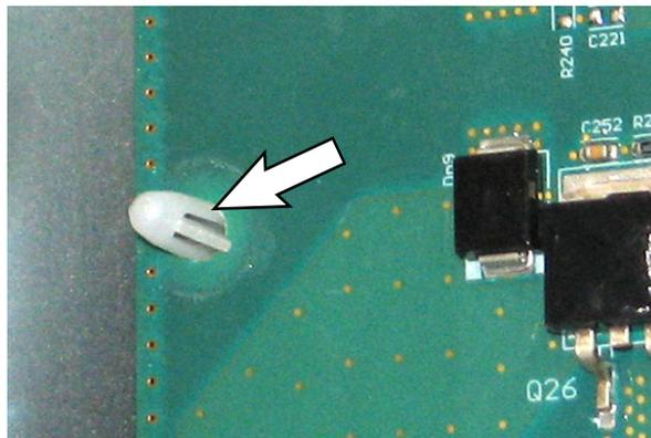
*NOTE: Replace damaged plastic standoffs. The standoffs secure the module into place and support the module away from the control housing. The standoffs must be replaced if damaged.*
