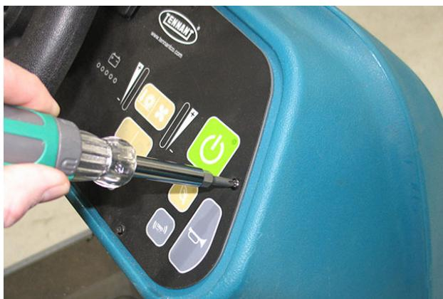
4. Carefully lift the membrane panel from the front shroud. Do not break any wire or cable connections when lifting the panel from the front shroud.
