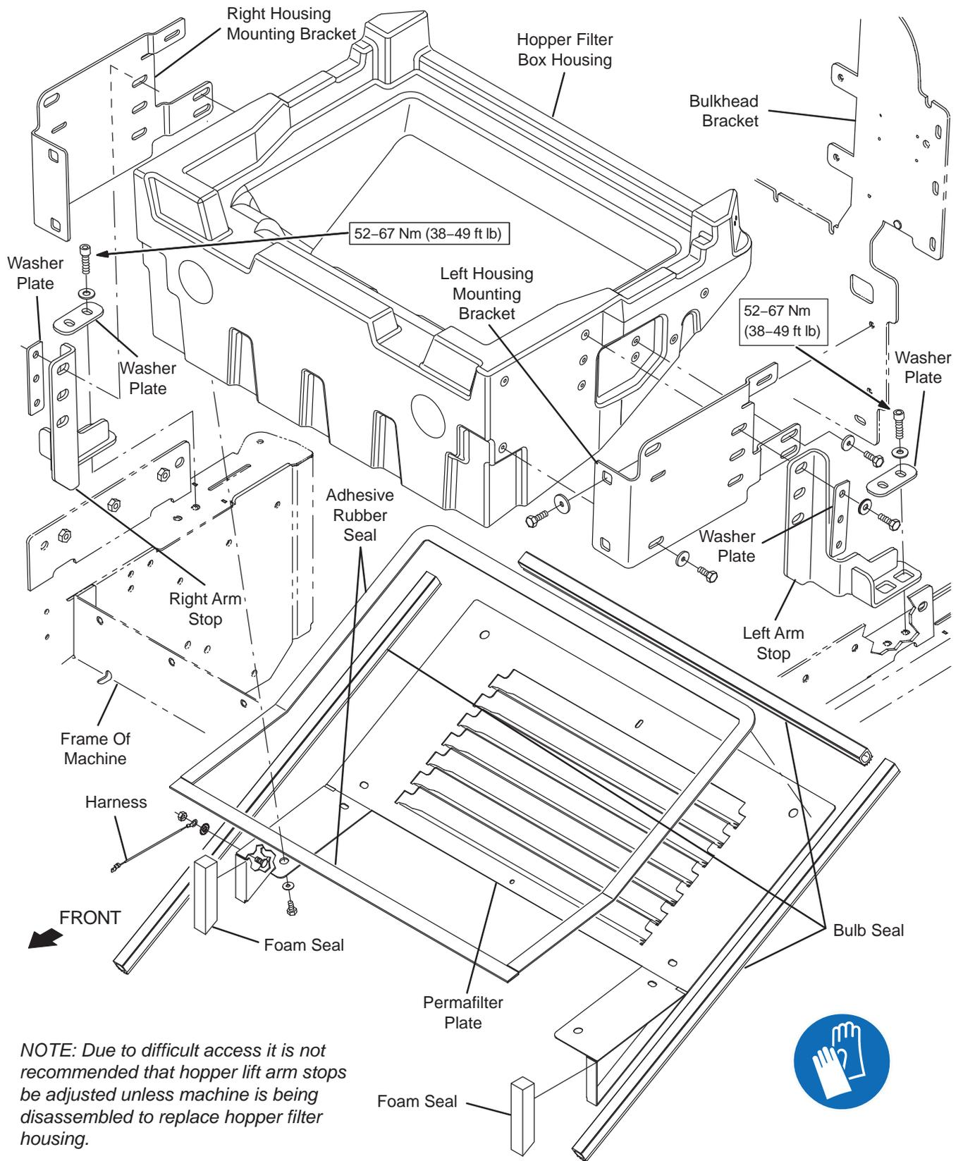
*NOTE: Due to difficult access it is not recommended that hopper lift arm stops be adjusted unless machine is being disassembled to replace hopper filter housing.*
