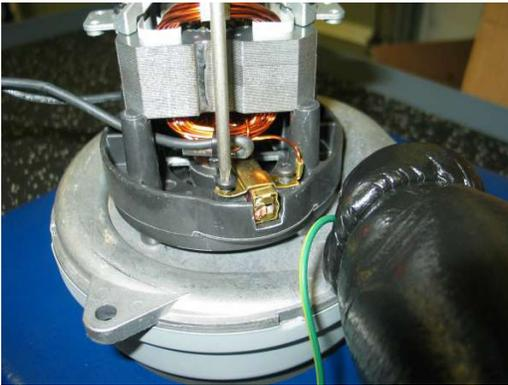
4. Lift up to release and remove carbon brushes from the vacuum fan motor.
