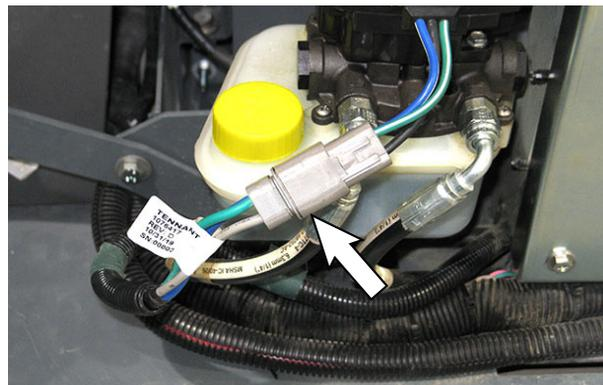
5. Mark/label the locations for the two hydraulic hoses connected to the hydraulic pump.
