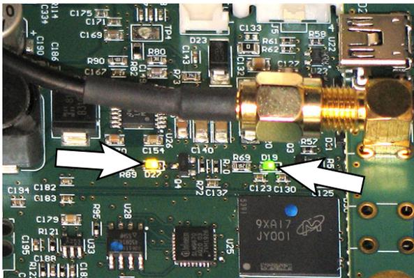
If no green micro-processor heartbeat LED indicator (D19), check for power at J7-10 on the main sweep circuit board.
