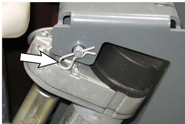
9. Install the new main sweep actuator/reinstall the removed actuator in the reverse order of disassembly.
