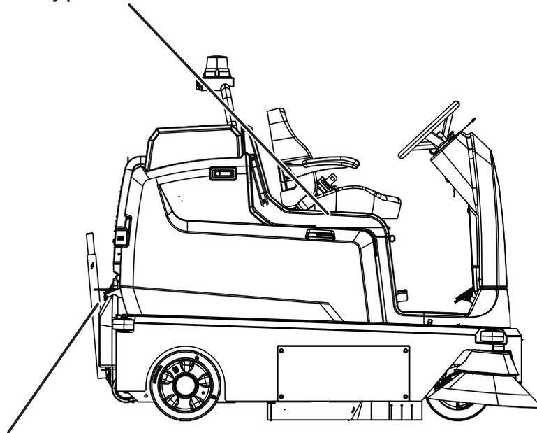
**WARNING LABEL - Brush throws debris. Stop motor before lifting hopper.**
