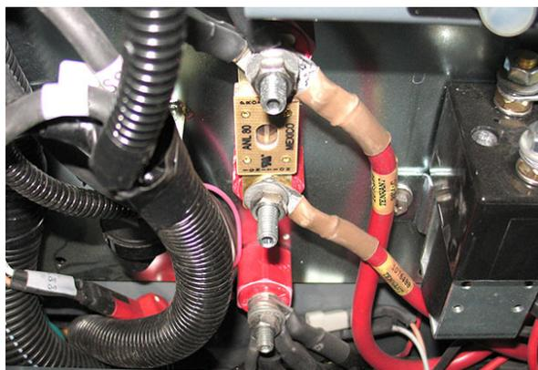
6. Inspect connections at Main Contactor (M1). Secure/repair connections. Continue testing/troubleshooting procedure if problem persists.
