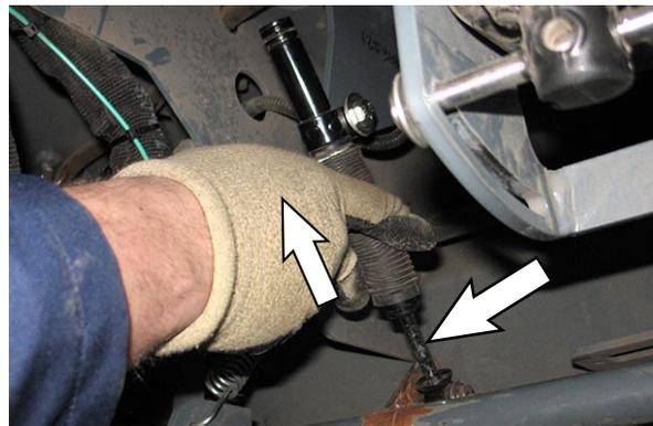
6. Inspect the shock absorber (damper) for damage/wear. Replace the shock absorber (damper) if damaged/worn.
