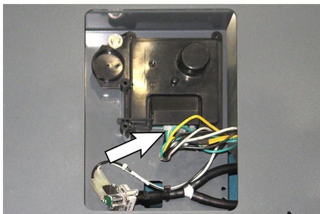
5. Remove the ABW controller from the ABW mounting bracket.
