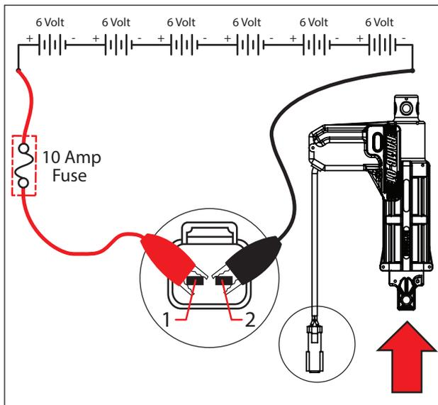
4. Reverse polarity and apply battery voltage to the lift actuator using fuse-protected jumper leads. Connect battery negative (-) to terminal 1 and battery positive (+) to terminal 2. The actuator should extend completely.
