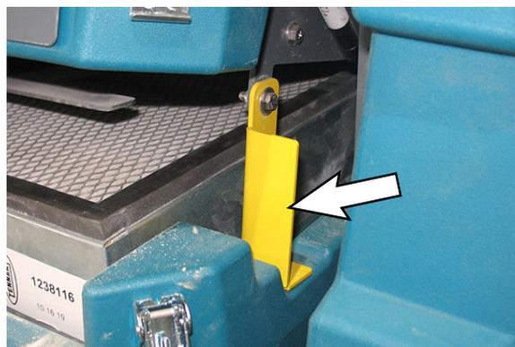
7. Remove the hopper filter from the hopper filter compartment.
