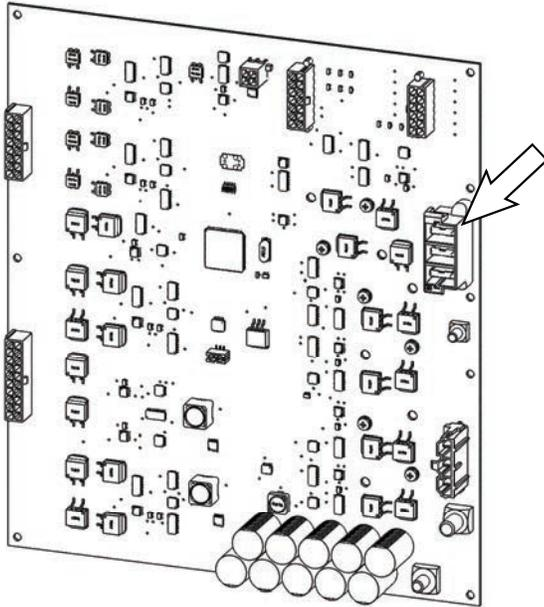
8. Check harness connections at the hydraulic pump. The coil resistance is typically less than  $0.5\Omega$  for both sides. J10-1 to J10-3 should measure less than  $0.5\Omega$  and J10-2 to J10-3 should measure less than  $0.5\Omega$ .
