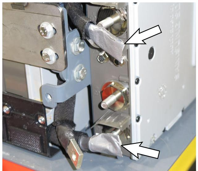
11. Remove the battery controller from the Lithium-Ion battery pack
