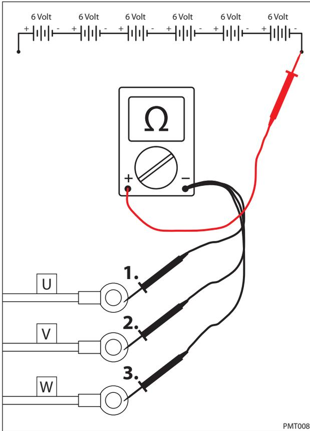
7. Test each cable using an ohmmeter for a short to chassis as shown below. Each cable should test as "O. L." or open to chassis.
