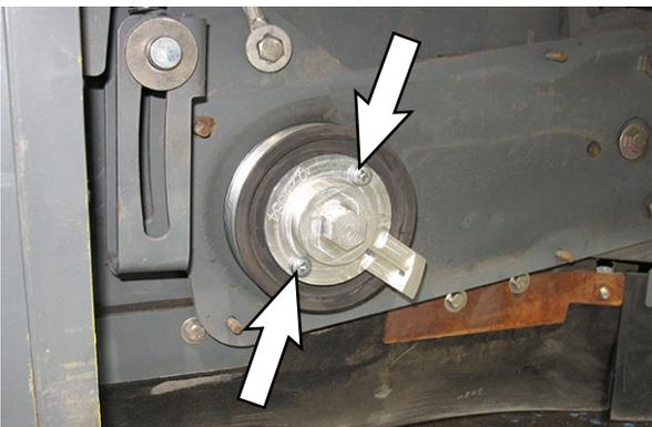
5. Position the belt onto the motor sheave and then position the belt onto the belt installation tool.
