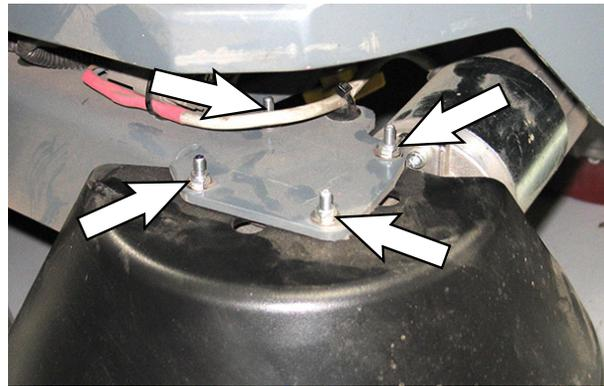
7. Remove the side brush guard from 36 VDC side brush motor.
