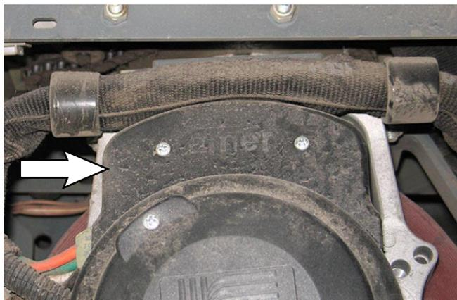
7. Disconnect the speed sensor cable and all main wire harness connections from the drive wheel assembly and encoder.
