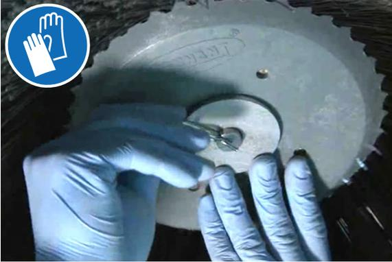
3. Remove the side brush and retainer from under the side brush assembly.
