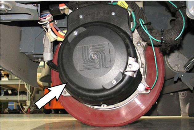
5. Remove the hardware securing the brake assembly to the drive wheel assembly. **Do Not** lose hardware securing the brake assembly. These parts will be needed to reinstall the brake assembly.
