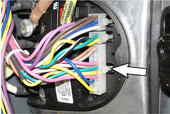
4. Check J1-15 and J1-16.  $62\Omega \pm 3\Omega$  at harness and  $120\ \text{ohm} \pm 5$  on the pins on Drive Controller (C3).
