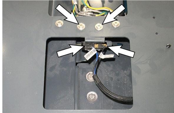
5. Remove the hopper position switch/switch mounting bracket from the right tower.
