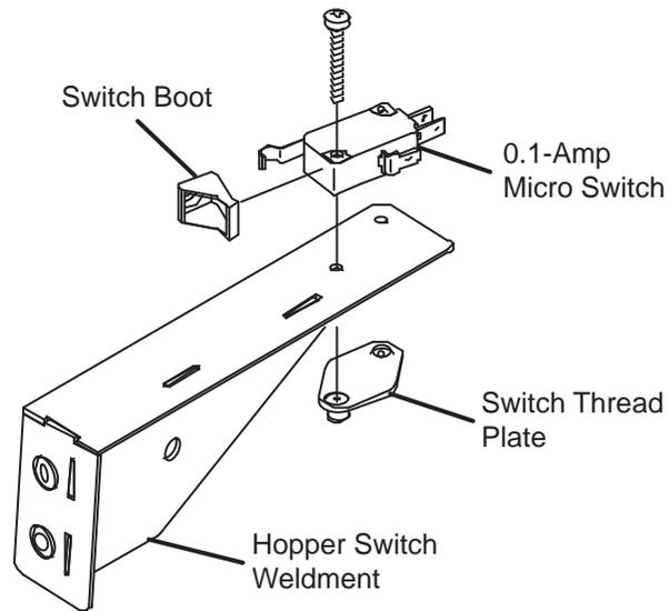
7. Install the new micro switch onto the hopper switch weldment.
