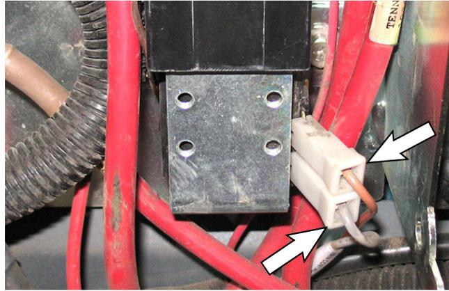
4. Disconnect wire harness connections from the top terminals of the contactor.
