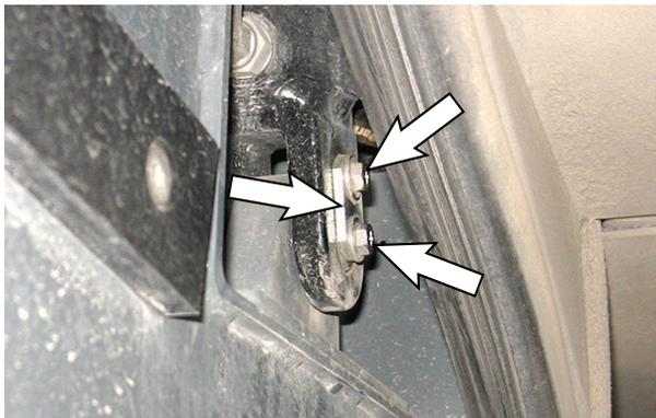
4. Remove the hardware and pin securing the top of the hopper hydraulic lift cylinder to the lower hopper arm and allow the hopper hydraulic lift cylinder to lower.
