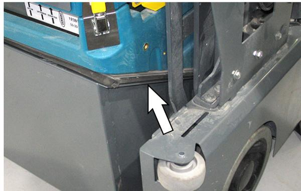
3. Loosen the hardware securing the adjustment plates to both the right tower and left tower.
