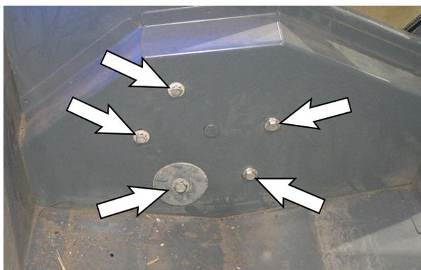
5. Tilt hopper back on the table so the front end of the hopper can clear the hopper lift components and pull the hopper out from the machine.
