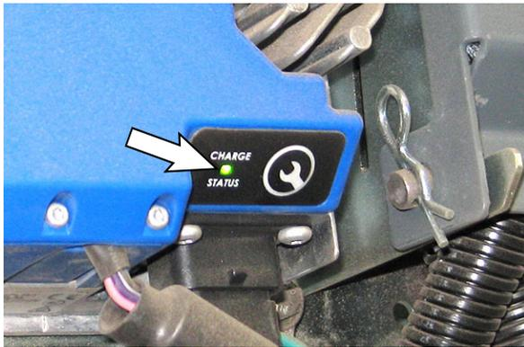
2. To enter the battery select mode to choose a new profile setting, press and hold the Select Charge Profile Button for 5 seconds. Fast red flashes will confirm select mode entry.
