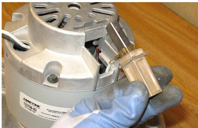
4. Disconnect the wire from the vacuum fan motor carbon brush.
