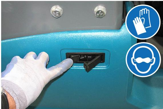
Periodically check the water level in the ABW tank. Add distilled water when low.
