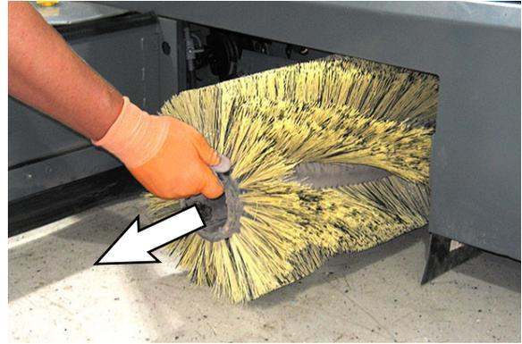
6. Put the new or rotated end-for-end main brush on the floor next to the main sweep compartment.
