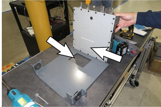
14. Apply blue thread sealant onto screws and reattach battery controller to bracket. Torque screws to 3.8 Nm +/- 0.7 Nm (2.8 ft lbs +/- 0.5 ft lbs).
