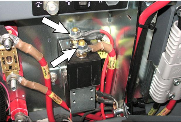
6. Remove the 200-A 36 VDC contactor from the charger mounting bracket.
