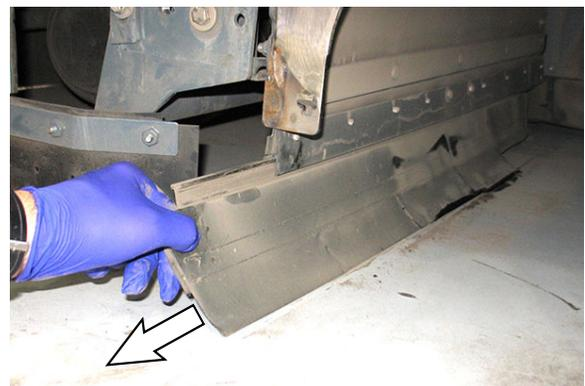
5. Install the new large debris trap skirt onto the sweep head.
