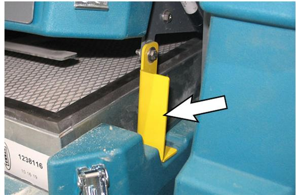
3. Remove the filter from the hopper filter compartment
