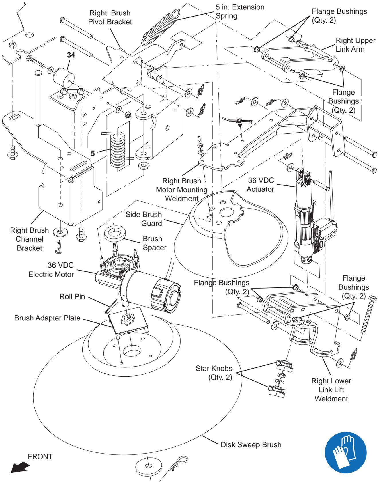
**NOTE:** This procedure can be used to remove/replace either the right side brush actuator or the left side brush actuator. Although only the standard right side sweep assembly is shown, the right side sweep illustration can be used for reference since all parts are located in same locations for the right side sweep assembly and the optional left side sweep assembly.
