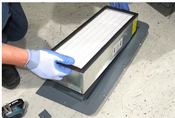
**NOTE:** Do Not touch or damage the new HEPA filter media when installing the HEPA filter onto the HEPA tray.
