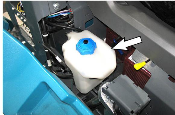
The automatic battery watering indicator will also alert user to add distilled water when tank is empty. See SMART-FILL ABW (AUTOMATIC BATTERY WATERING) INDICATOR.
