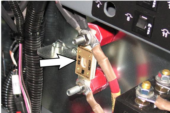
The fuses are located in the control box behind the circuit breaker panel or in-line on harnesses and cables.
