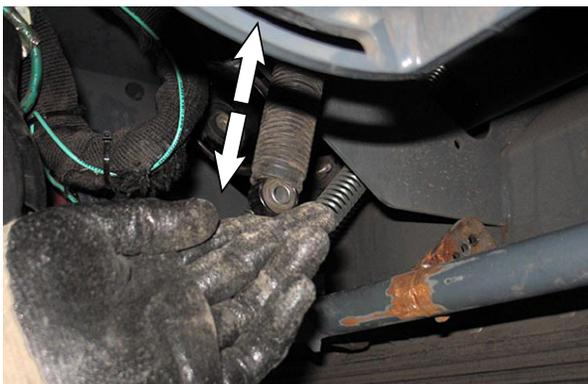
11. If the shock absorber (damper) is not damaged, passes the brush bounce test and the manual test the shock absorber (damper) does not need to be replaced. Reinstall the previously removed M6 shoulder screw to secure the shock absorber (damper) to the sweep lift arm.
