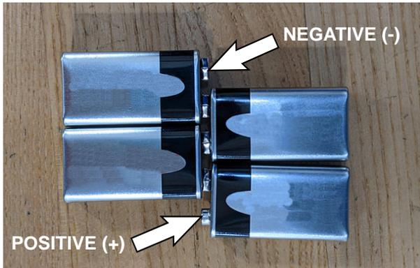
2. Wrap tape around batteries to stabilize the battery pack, leaving the unconnected positive and negative terminals exposed.
