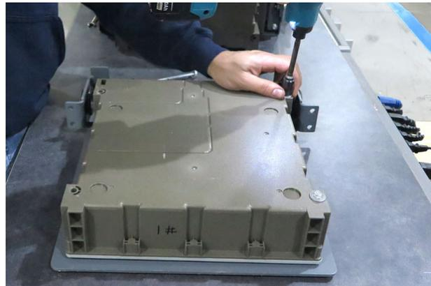
15. Install the battery controller onto the Lithium-Ion battery pack in reverse order of disassembly.
