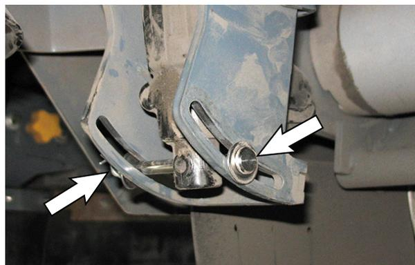
7. Remove the hardware securing the 36 VDC actuator to the brush pivot bracket.
