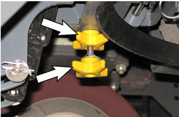
3. Turn key switch ON, completely lower the side brush to allow access to all side brush motor mounting hardware, and turn the key switch OFF.
