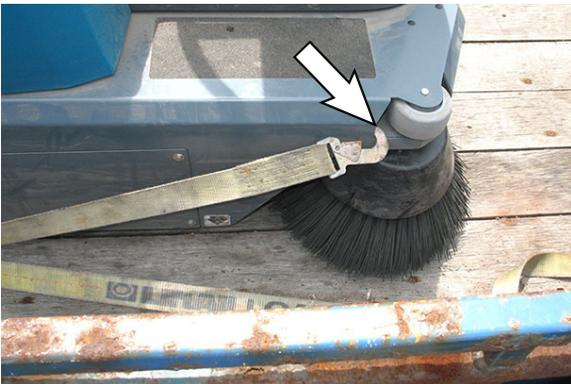
If machine is equipped with the optional dust control skirts, connect the tie down straps to the holes in the bumper wheel brackets located on each side of the machine to secure the machine to the truck or trailer.
