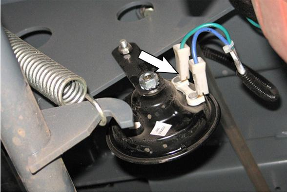
2. Read voltage across horn while horn button is pressed. If voltage is not ~19V to 23V (when battery is between 31.5V and 38V), check wires and connections for damage.
