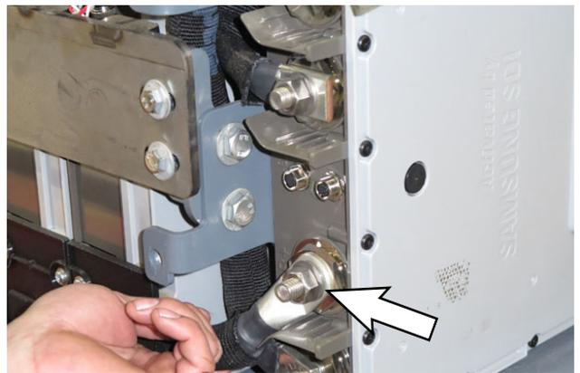
10. Wrap the Lithium-Ion battery pack cable connectors with tape to prevent the cables from arcing.
