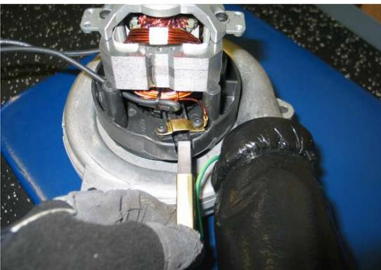
5. Inspect carbon brushes. Replace carbon brushes if they are stuck or are less than 10 mm (0.375 in) in length.
