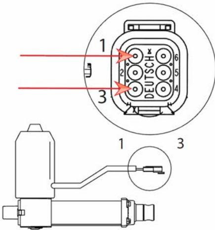
3. Use fuse-protected jumper leads to apply battery voltage to the actuator. Connect battery positive (+) to terminal 1 and battery negative (-) to terminal 3. The actuator should extend completely.
