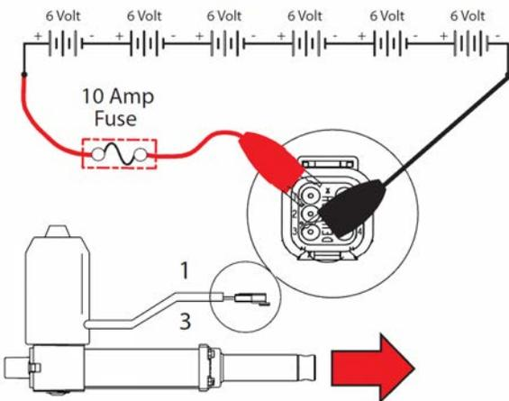
4. Use fuse-protected jumper leads to apply battery voltage to the roll out actuator. Connect battery positive (+) to terminal 3 and battery negative (-) to terminal 1. The actuator should retract completely.
