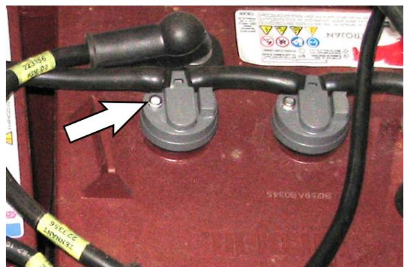
6. After adding water, reinstall the dust cap onto the battery fill hose and store the hand pump hose inside the battery compartment for future use.
