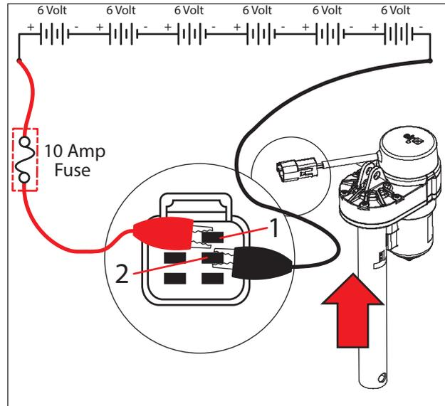
4. Use fuse-protected jumper leads to reverse polarity and apply battery voltage to the lift actuator. Connect battery negative (-) to terminal 1 and battery positive (+) to terminal 2. The actuator should extend completely.
