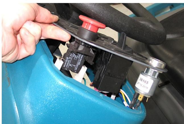
5. If removing the console to conduct other service/maintenance disconnect all wire harness connections from the controls installed on the panel.
