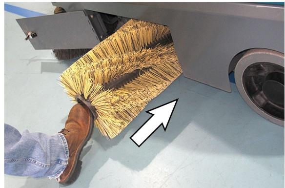
8. Reinstall the idler arm assembly onto the main sweep assembly. Be sure to keep the idler arm above the brush compartment skirt when installing the idler arm assembly onto the main sweep assembly.
