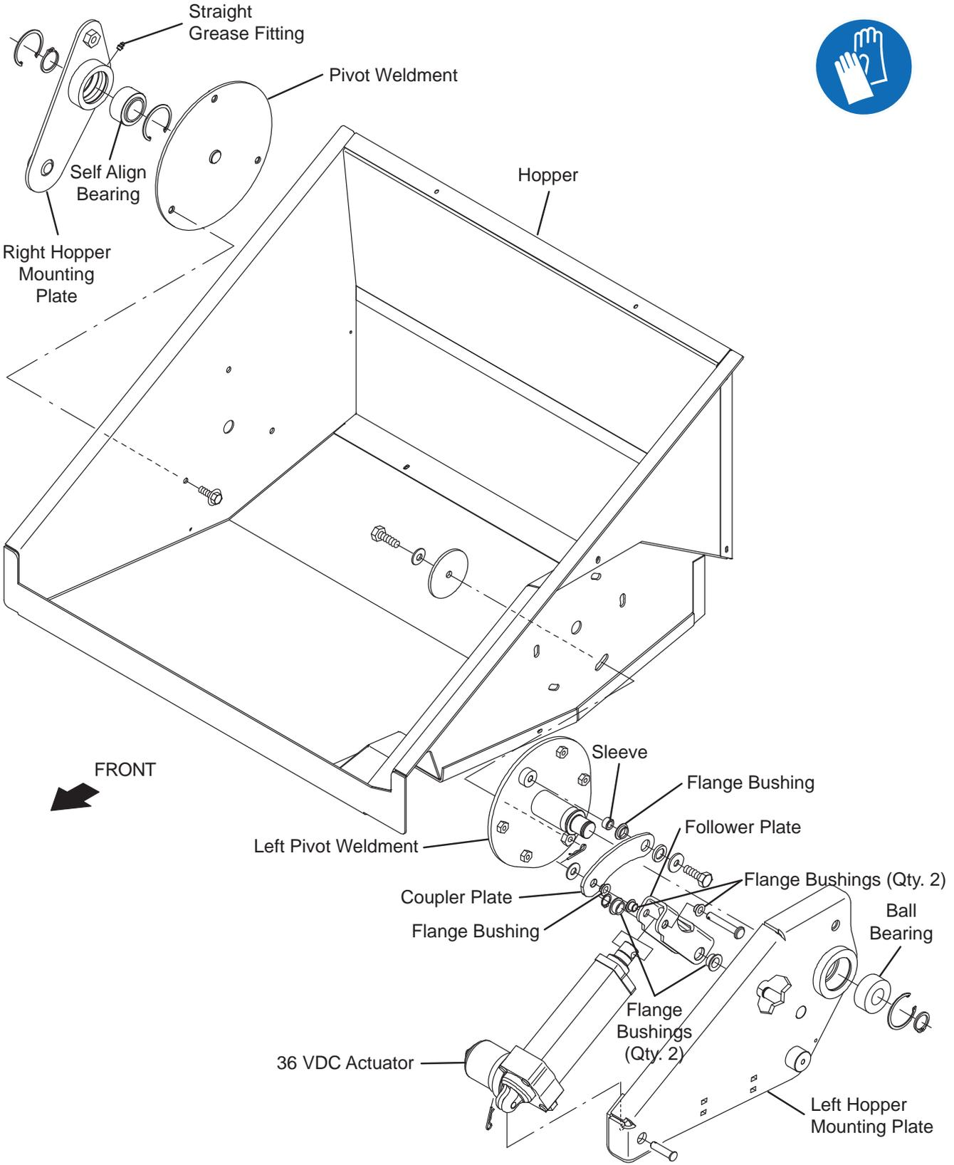
1. Turn the key switch ON, and raise the hopper approximately half way, turn the key switch OFF, and remove the key.
