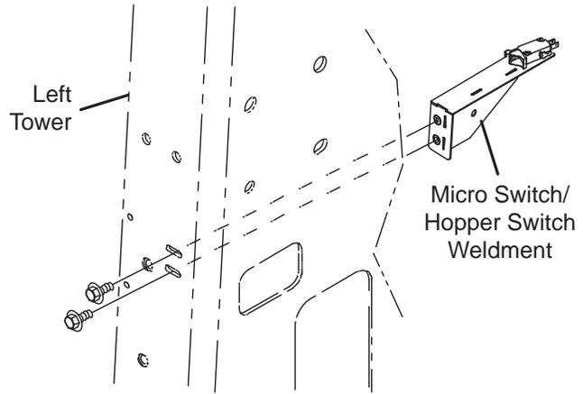
6. Remove the micro switch from the hopper switch weldment.
