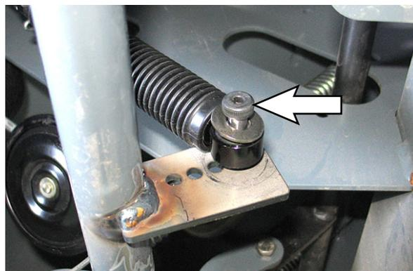
11. Remove hardware securing the sweep lift arm to the pivot mounting bracket and the left pivot mounting bracket and remove the sweep lift arm from under the machine.
