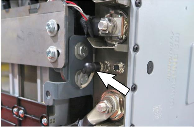
*NOTE: If Lithium-Ion battery pack is equipped with two COM cables, disconnect both COM cables from the battery controller.*
