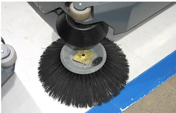
2. Loosen the top star knob and turn the bottom star knob clockwise until it is at the position for a new or moderately worn brush.
