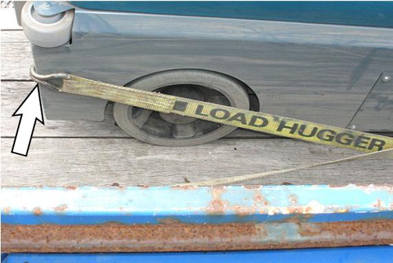
9. Connect the tie-down straps to the front of the frame of the machine, in the recessed area located on both sides of the machine directly behind each front bumper wheel and secure the tie-downs to the trailer or truck to prevent the machine from moving.
