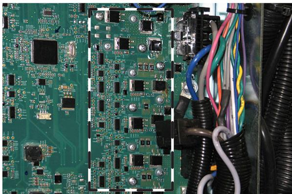
6. Carefully squeeze the plastic standoffs (Qty. 4) located at each corner of the main sweep circuit board to release the circuit board from the electrical enclosure panel and remove the main sweep circuit board from the enclosure.
