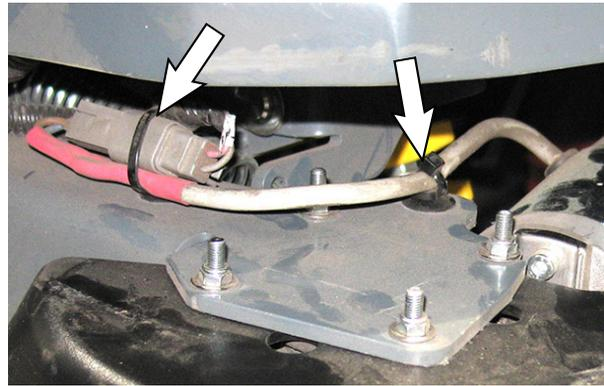
6. Remove the hardware securing the 36 VDC side brush motor and side brush guard to the brush motor mounting weldment.
