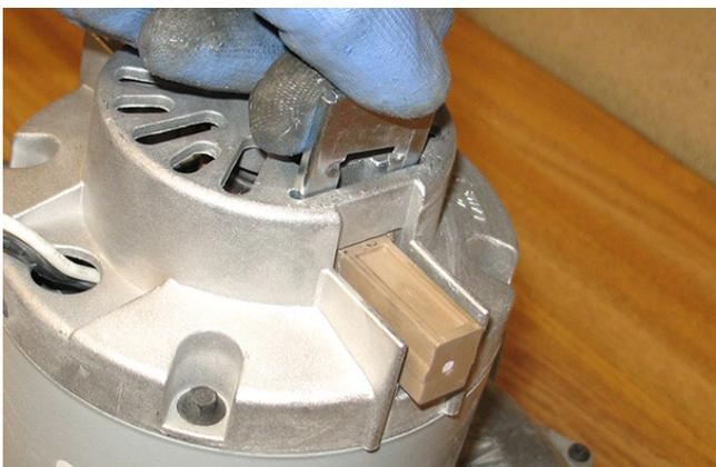
3. Carefully pull the carbon brush from the vacuum fan motor.
