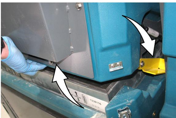
**NOTE: Ensure the hopper filter compartment prop arm is fully engaged before removing the filter from the machine.**
