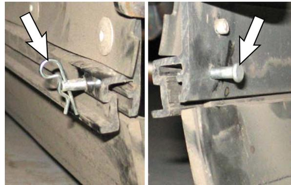
4. Pull the large debris trap skirt from the sweep head.
