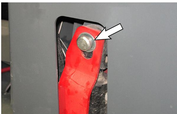
5. Carefully pull the hopper hydraulic lift cylinder out toward the rear of the machine.
