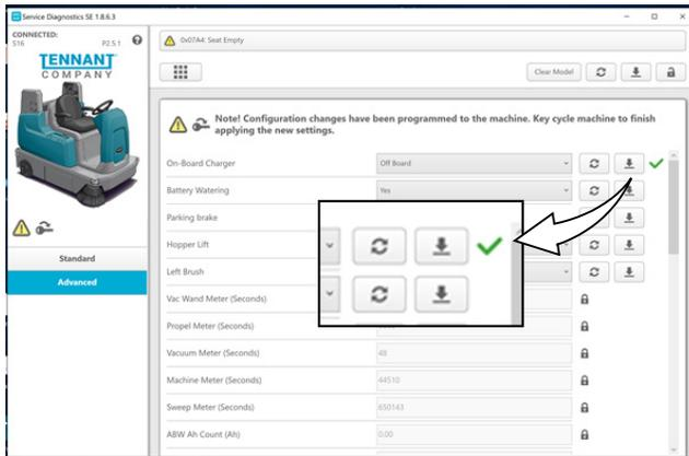
Cycle the key switch to save the new advanced configuration setting(s). That setting(s) will not be saved until the machine is key cycled.
