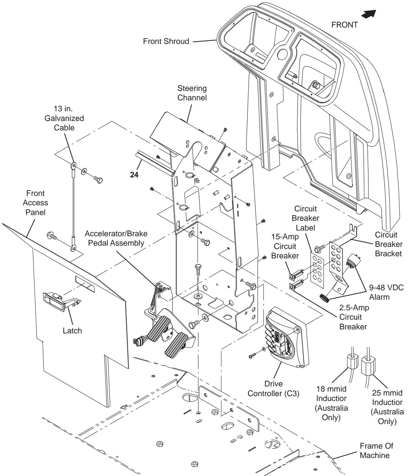
\*NOTE: Be sure all connectors on propel cable assembly are connected to corresponding locations on Drive Controller (C3). Refer to labels on propel cable assembly and markings on Drive Controller (C3).
