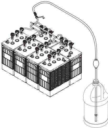
The optional manual battery watering system provides a safe and easy way to maintain the proper electrolyte levels in your batteries. It is designed exclusively for flooded (wet) lead-acid batteries.
