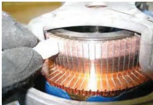
7. Use compressed air to clean dust from inside the vacuum fan motor.
