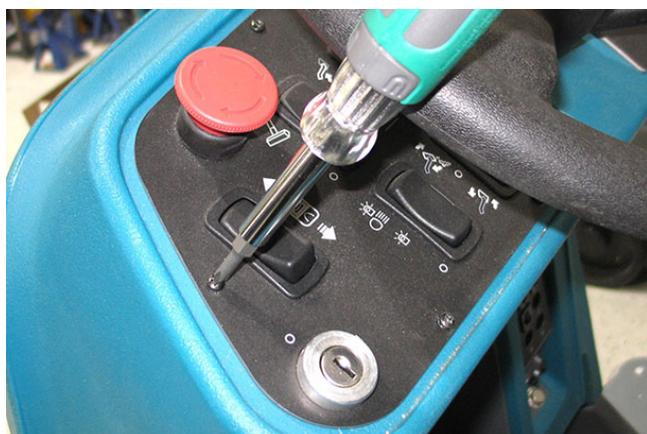
4. Carefully lift the control panel from the shroud. Do not break any wire or cable connections when lifting the panel from the front shroud.
