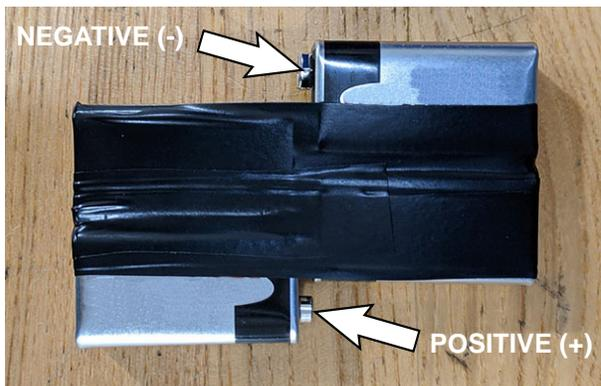
**NOTE:** This battery pack is only meant for brief 1-2 second testing. The battery pack cannot sustain large currents.
