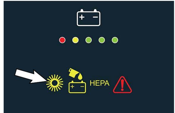
**NOTE:** Types of brush condition, floor surfaces, debris being swept, brush pressure, and any combination of the four can affect whether the worn brush indicator illuminates. The indicator could illuminate while machine is sweeping lighter debris or a smoother surface, and then go off when the machine is sweeping heavy debris or on a rough surface. Adjusting the brush pressure can also affect when the indicator illuminates, or goes off if already illuminated.
