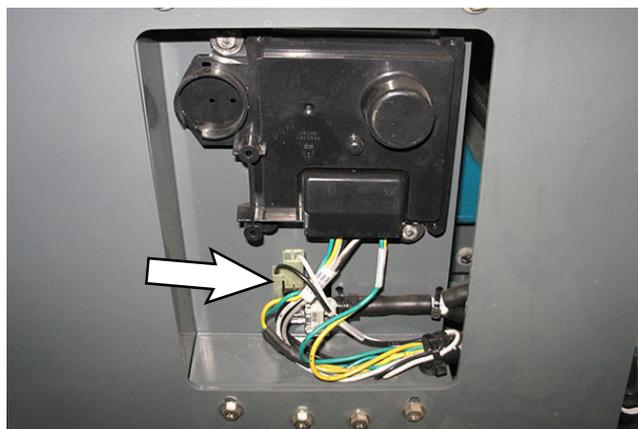
6. Cut the cable ties securing the battery water delivery assembly to the ABW mounting bracket.
