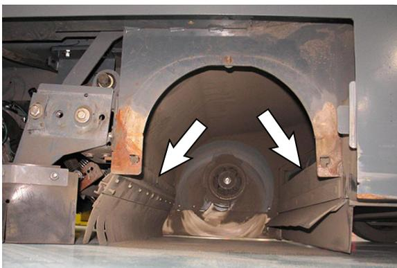
Check the brush pattern and rotate the brush end-for-end after every 50 hours of operation, for maximum brush life and best sweeping performance. Refer to *REPLACING OR ROTATING THE MAIN BRUSH*.
