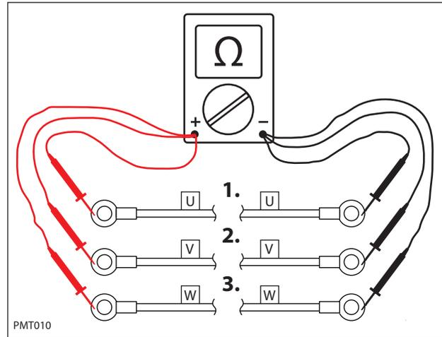
9. "Tug test" each cable (motor end) to determine if a cable is broken inside the insulation. Do not exceed 10 lbs (45 N) of force as cable damage may occur.
