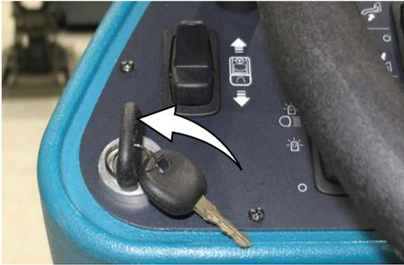
2. Press and hold the center of the 1-Step button and turn the key switch ON.
