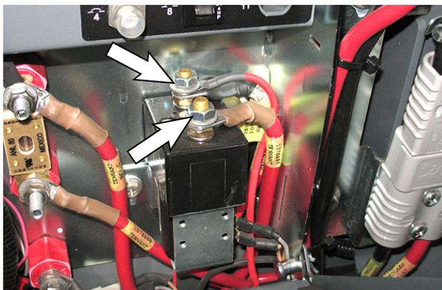
6. Disconnect the connector from one of the coil terminals located on the lower side of the main contactor (M1).
