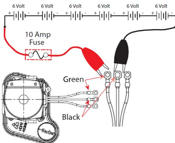
4. Use fuse-protected jumper leads to apply battery voltage to the pump motor. Connect battery positive (+) to blue wire and battery negative (-) to black wire. The motor should engage hydraulic cylinder to raise.
