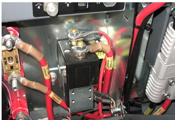
6. Confirm connections at B- and B+ main sweep circuit board. Secure/repair connections.
