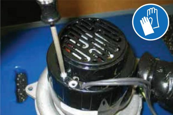
3. Loosen the carbon brush mounting hardware.
