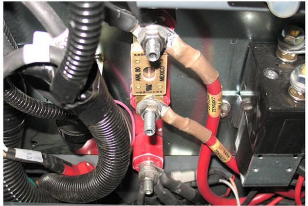
6. Inspect connections at Main Contactor (M1). Secure/repair connections. Continue testing/troubleshooting procedure if problem persists.
