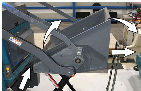
6. Install the new hopper/reinstall the removed hopper onto the machine in reverse order of disassembly.
