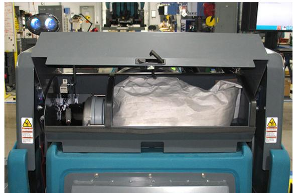
3. Remove the vacuum wand bag from the vacuum wand compartment.
