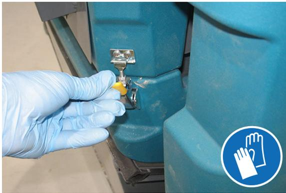
2. Lift the hopper filter compartment until the hopper filter compartment prop arms secure the hopper filter compartment open.
