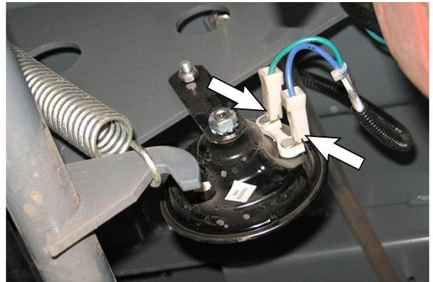
6. Ensure main harness wires to the horn are not damaged (pinched, discolored, etc...).
