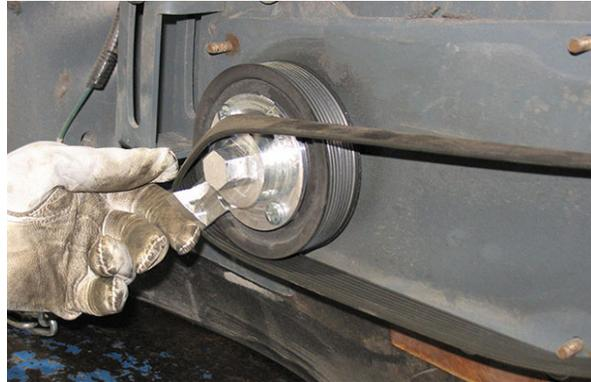
6. Turn the belt installation tool/sheave clockwise to install the belt onto both sheaves.
