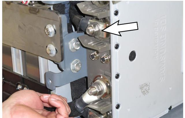
Disconnect the positive (+) terminal after the negative (-) has been disconnected.
