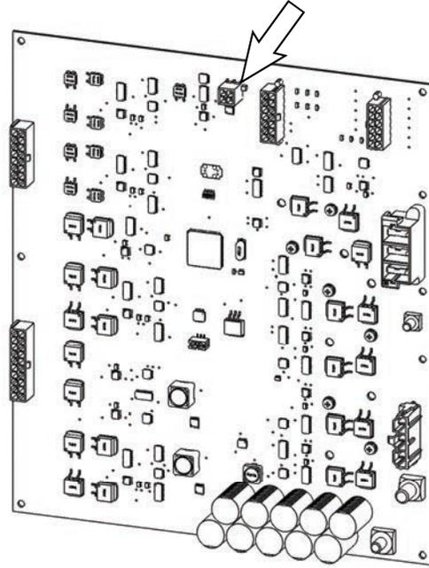
Measure between yellow and green on harness and should be  $61\Omega \pm 2\Omega$ .
