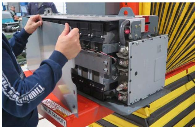
7. Disconnect the Lithium-Ion battery pack control cable and COM cable from the battery controller.
