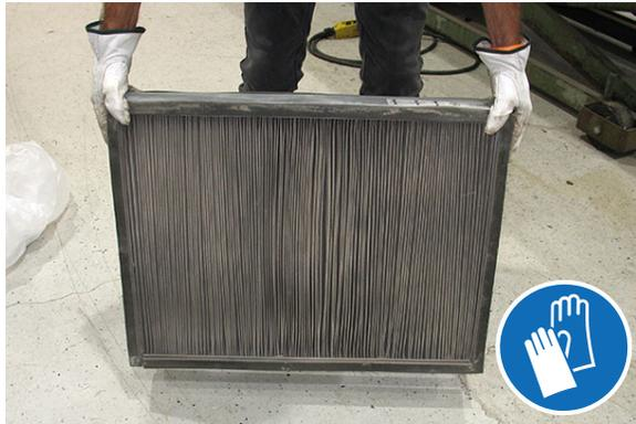
**AIR**-Always wear eye protection when using compressed air. Blow air through the center of the filter and out toward the exterior. Never use more than 550 kPa (80 psi) of air pressure with a nozzle no smaller than 3 mm (0.13 in) and never hold the nozzle closer than 50 mm (2 in) to the filter.
