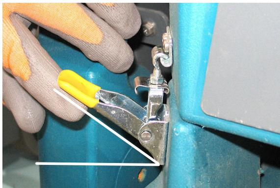
3. Leave the latch hook still attached to the latch keeper, and turn the jam nut to shorten the latch length.
