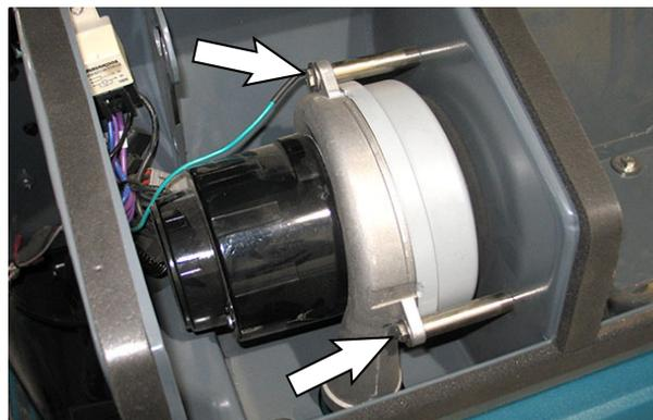
10. Remove the vacuum wand fan motor from the filter box.
