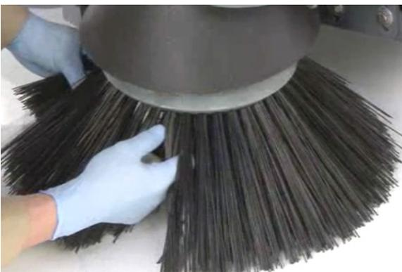
4. Place the side brush underneath the side brush assembly and align the channel in the retainer with the retainer pin in the side brush hub.
