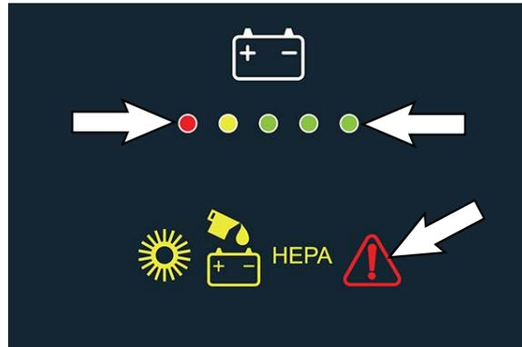
To reset the fault/alert indicators, turn off the machine and eliminate the cause of the fault/alert. The fault/alert and will reset when the machine is again turned on.
