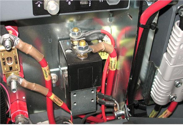
11. Confirm connections at B- and B+ main sweep circuit board. Secure/repair connections to main sweep circuit board as necessary.
