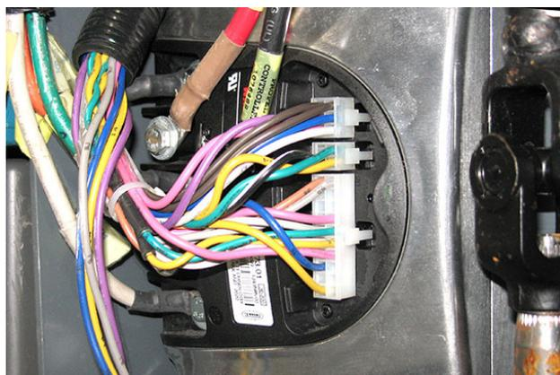
5. Remove the hardware securing the drive controller (C3) to the steering channel.
