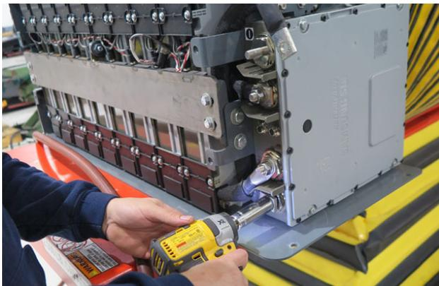
9. Disconnect the Lithium-Ion battery pack bus cables from the battery controller. Disconnect the negative (-) terminal connection first.
