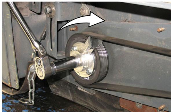
7. Rotate the belt on the sheaves and use fingers to work the belt the rest of the way onto the sheaves
