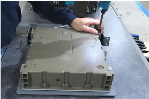
13. Reassemble the bracket onto the battery controller. Be sure the protruded area on the battery controller goes back into the cut out section in the bracket.
