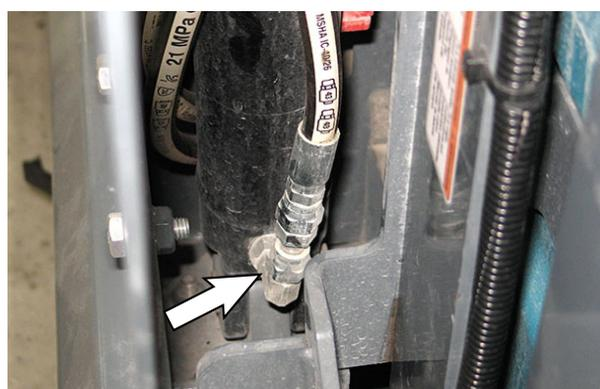
7. Mark each hose with location it was removed from the hopper hydraulic lift cylinder.
