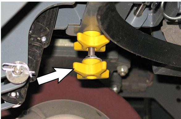
4. Tighten the upper star knob to secure the side brush pattern adjustment.
