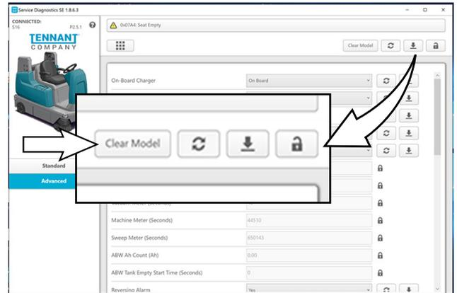
14. A warning box appears stating "Warning! Machine configuration and model information are going to be erased. After this is complete, you will be required to reconfigure machine through the new board wizard. Are you sure you want to do this?" Select the Yes button to continue complete reconfiguring the machine.
