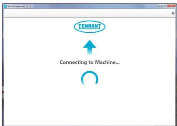
5. The Service Diagnostics tool automatically detects a new interface module installation if a new interface module was installed. Enter the model and serial number and then click the arrow button.
