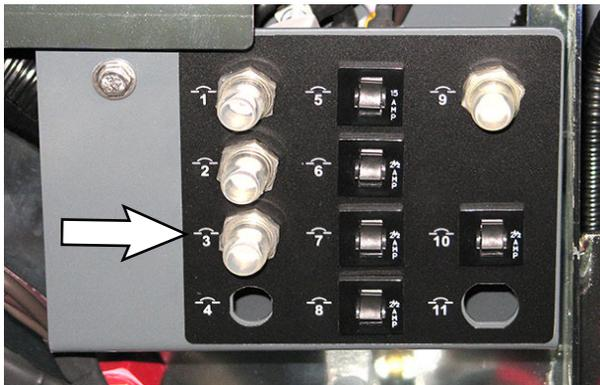
5. Check in-line 100-Amp fuse. Secure/repair connections. Continue testing/troubleshooting procedure if problem persists.
