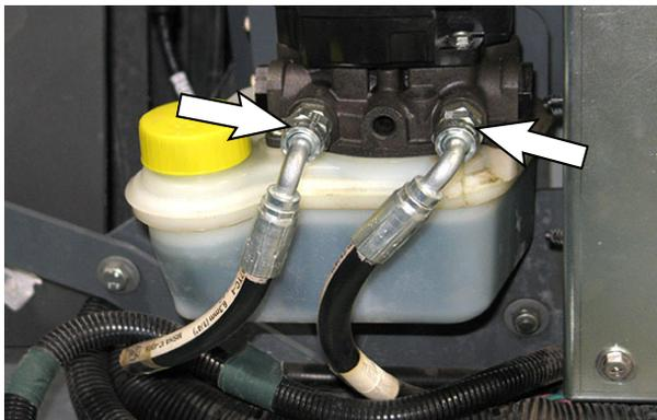
6. Disconnect the hydraulic hoses from the hydraulic pump and cap the ends of the hoses to prevent hydraulic fluid from escaping from the hydraulic system.
