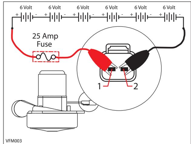
5. Reconnect vacuum fan(s) to wire harness. See *MANUAL MODE*. Activate the vacuum fan in Manual Mode. The amperage displayed should be approximately 14-20 Amps (average 16 Amps).
