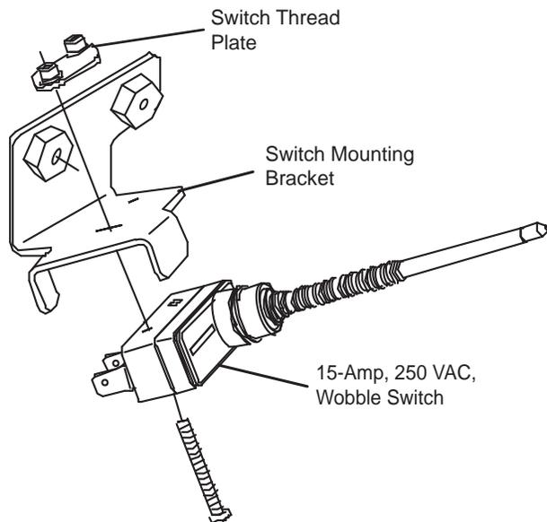
7. Install the new hopper position switch onto the switch mounting bracket.
