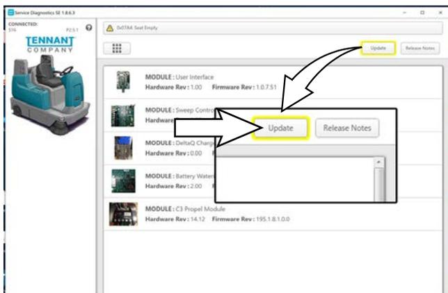
The process indicator will disappear from the screen and all items in the firmware update status bar will have check marks to the left to verify the firmware has occurred.
