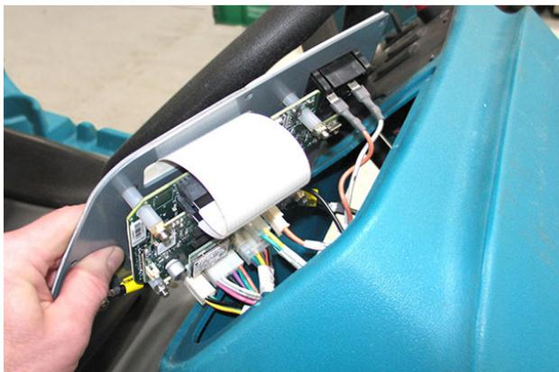
5. If completely removing the membrane panel/ replacing the membrane panel, disconnect all wire and cable connections from the panel .
