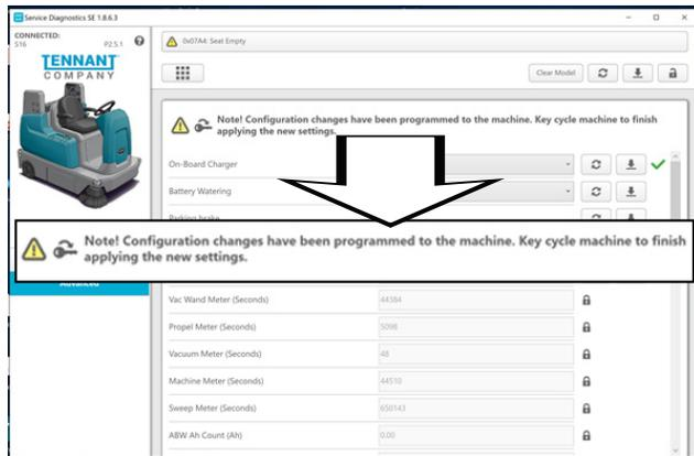
13. If the machine must be completely reconfigured, select the Clear Model button to completely clear all previous machine configuration parameters and completely reconfigure the machine.
