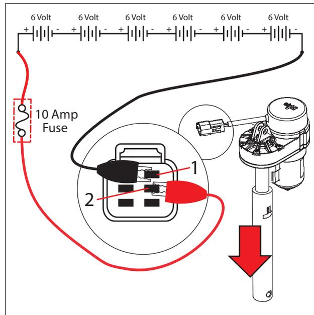
**TESTING THE SWEEP/HEPA VACUUM FAN**
