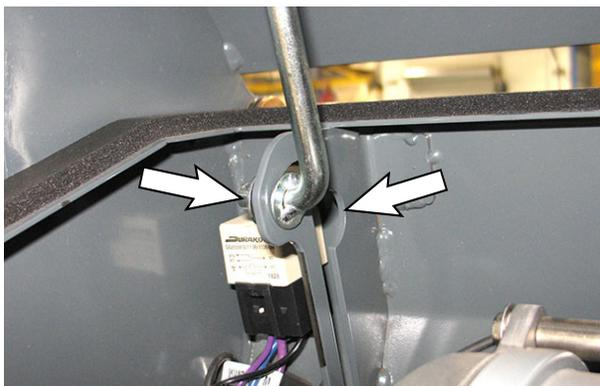
*NOTE: The torsion spring installed on the other end of the support safety arm will cause the support safety arm to snap quickly to the filter box cover. Use care when disengaging the support safety arm from the filter box.*
