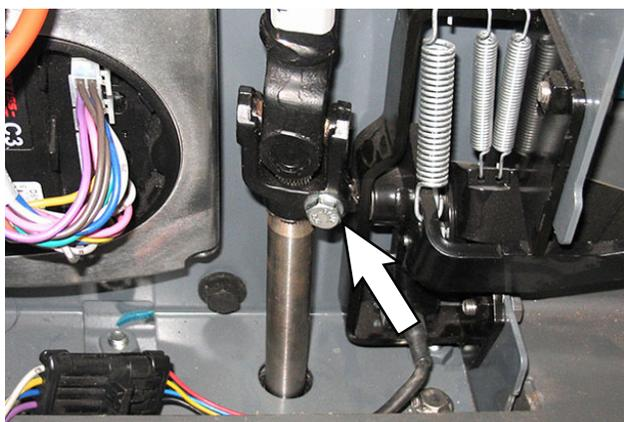
4. Lift the u-joint from the steering control assembly shaft.
