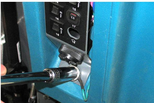
*NOTE: To avoid damaging electronic components, a static ground strap must be worn at all times while handling/testing electrical components. Attach the other end of the static ground strap to the machine chassis.*
