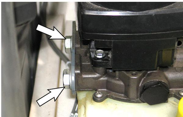
8. Install the new hydraulic pump onto the machine reverse order of disassembly.
