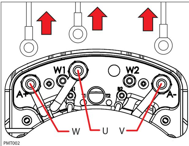
4. Use an ohmmeter to test the resistance of all three motor windings. The resistances of each winding should not be open (O. L.). An open winding indicates a faulty motor.
