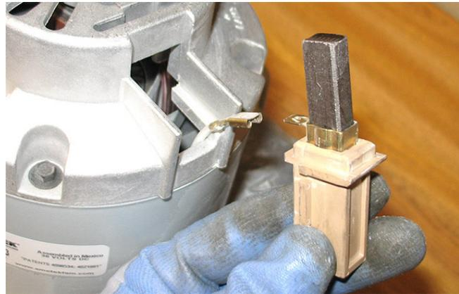
5. Inspect carbon brushes. Replace carbon brushes if they are stuck (brush should freely extend/retract in holder) or are less than 0.375 in. (10 mm) in length.
