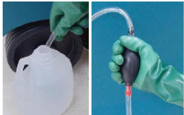
5. Squeeze the bulb on the hand pump hose until firm. The level indicators will turn white when full.
