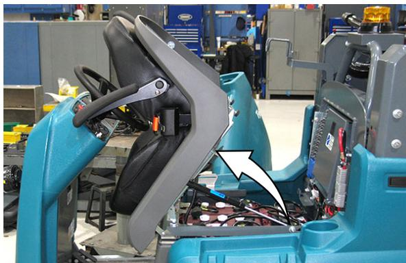
Open the electrical compartment cover to access circuit breakers 1 through 11.
