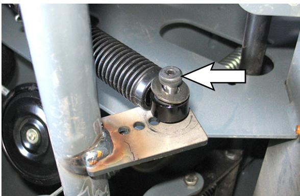
10. Use hand to extend and retract the shock absorber (damper). The shock absorber (damper) should remain in position when not being moved by hand, and always resist motion. If there is no resistance when retracting/extending the shock absorber (damper), or it does not remain in position when released, replace the shock absorber (damper).
