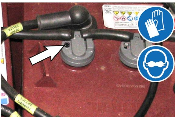
3. Locate the battery fill hose coupler inside the battery compartment. Remove the dust cap and connect the hand pump hose.
