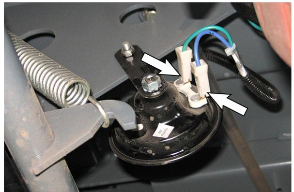
8. Check the pins for shorts (possibly due to moisture/debris between pins).
