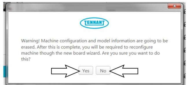
Select the No button to cancel complete machine configuration and return to Advanced configuration screen.
