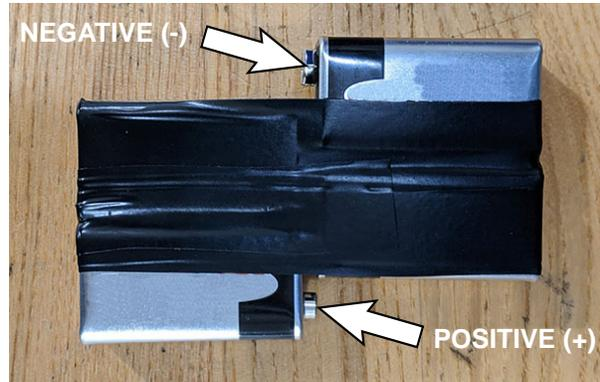
17. Touch (do not connect) the second alligator clip to the NEGATIVE (-) battery pack terminal and watch for the actuator to move.
