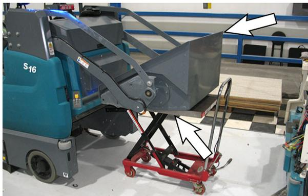
3. Turn the key switch ON, lower the hopper onto item being used to support the hopper, turn the key switch OFF, and remove the key.
