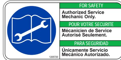
Located on electronic compartment cover (behind operator seat shroud).
