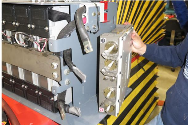
12. Remove the bracket from the battery controller.
