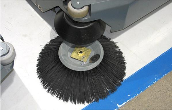
2. Loosen the top star knob and turn the bottom star knob counterclockwise until it is at the position for a completely worn brush.
