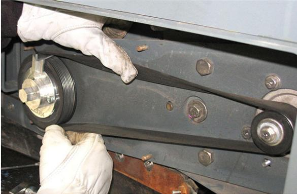
8. Remove the belt installation tool from the sheave.
