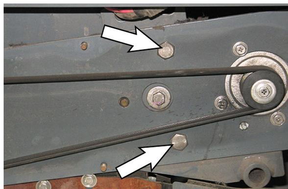
9. Remove the drive weldment from the machine.
