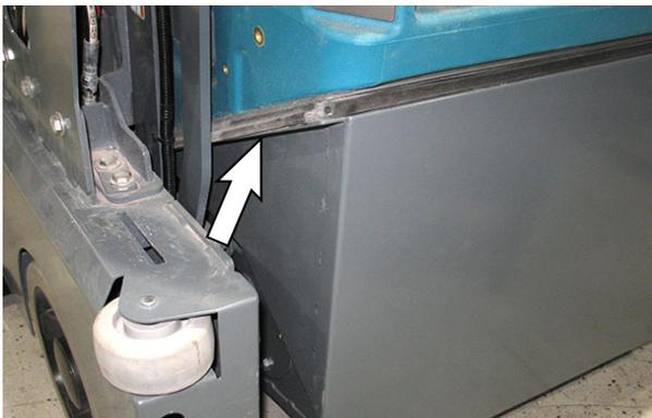
If the hopper edge is not parallel with seal plate, proceed to the following step to adjust pitch.
