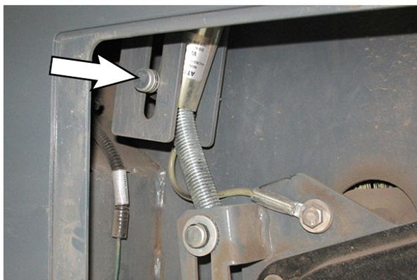
8. Remove the clevis pin/cotter pin securing the actuator to the sweep actuator mount.
