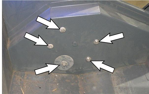
6. Adjust the hopper so the edge of the hopper is parallel with the top edge of the left hopper mounting plate.
