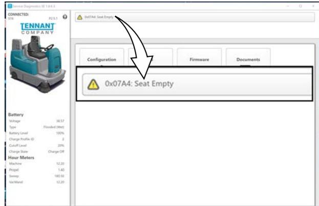
5. If faults are shown or the horn does not function, troubleshoot for a CAN and Main Sweep Module issue.
