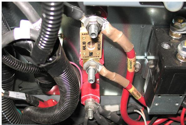
5. Inspect connections at Main Contactor (M1). Secure/repair connections. Continue testing/troubleshooting procedure if problem persists.
