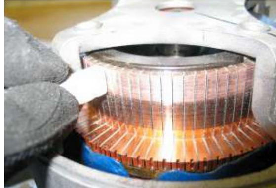
7. Use compressed air to clean dust from inside the vacuum fan motor.
