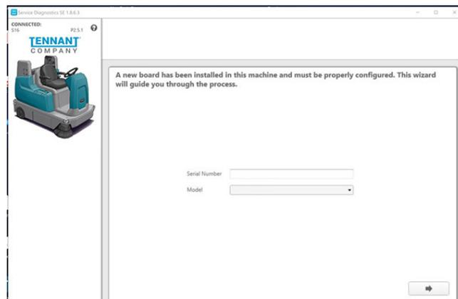
6. Inspect the actual machine configuration and match applicable configurations from the drop-down menus and then click on the arrow button.
