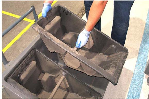
6. Reinstall the hopper into the machine.
