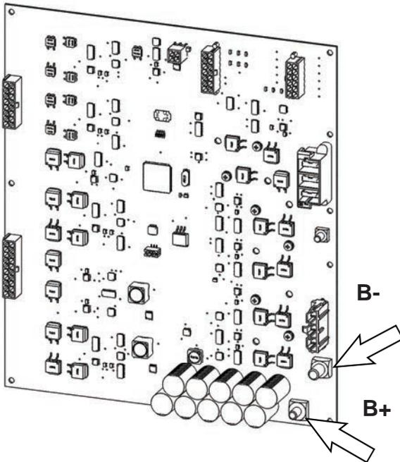
12. Reconnect the battery cable to the machine.
