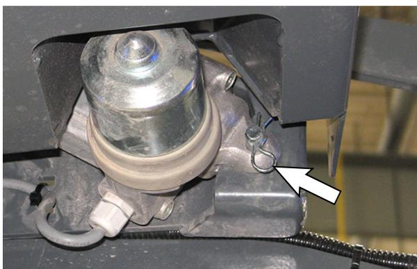
6. Remove the cotter pin securing the clevis pin in the rollout actuator and follower plate
