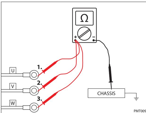
8. Use an ohmmeter to test each cable for end-to-end continuity. Each cable should test between 0-1 $\Omega$  resistance.
