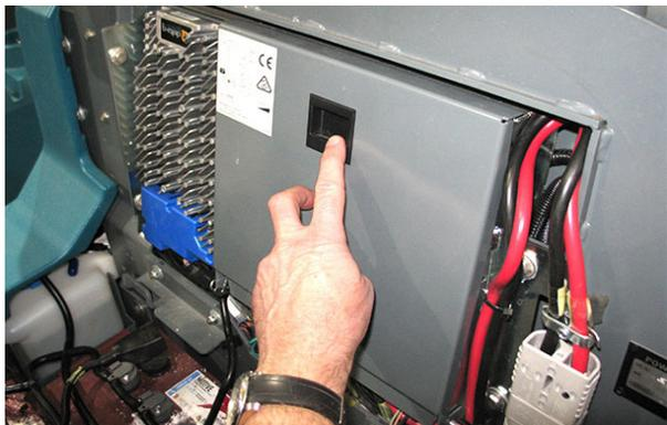
5. Ensure hardware securing connections to the terminals on top of the main contactor (M1) are tight.
