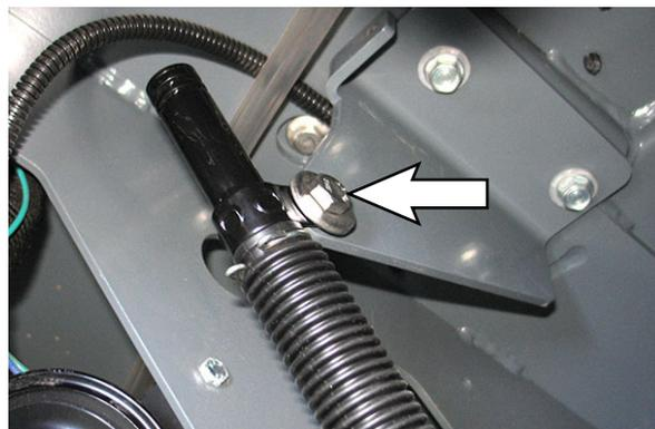
13. Install the new shock absorber (damper) in reverse order of disassembly.
