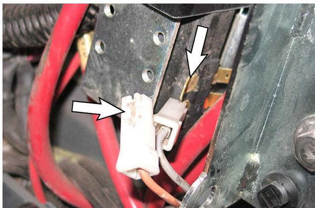
7. Test/confirm resistance across main contactor coil terminals (approximately 92-112Ω).
