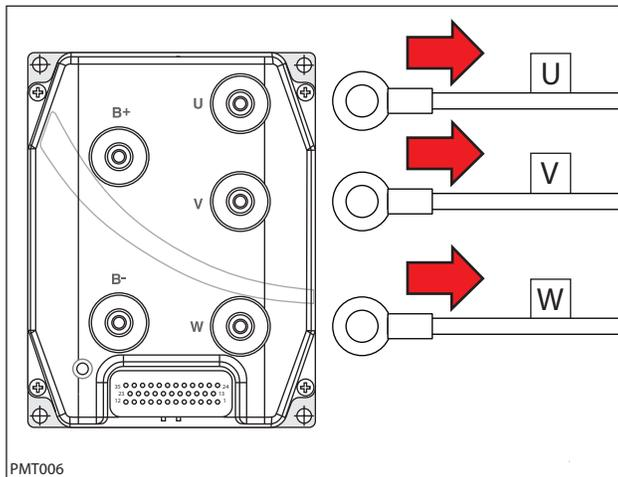
5. Reconnect battery connection and test each cable using an ohmmeter for a short to battery +. Each cable should test as "O. L." or open to battery +.
