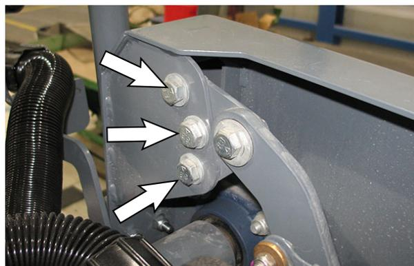
4. Place a floor jack under the back edge of the hopper and raise the jack enough to raise/adjust the hopper position so the hopper is pressed evenly at between 0.75 in. and 0.875 in. (19 mm and 22 mm) on each bulb seal installed on the bottom of the hopper filter box housing.
