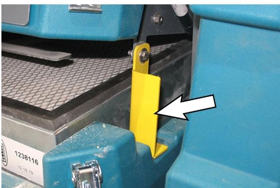
5. Remove the filter from the hopper filter compartment.
