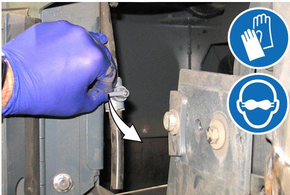
3. Close the battery compartment drain valve after all liquid has drained from the battery compartment.
