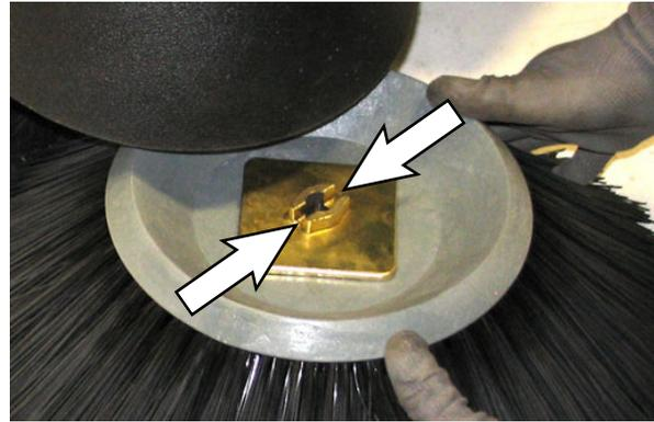
5. Lift the side brush, retainer, and washer up onto the side brush hub and reinstall the cotter pin into the hub.
