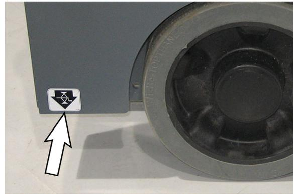
**FOR SAFETY:** When servicing machine, block machine tires before jacking machine up. Use a hoist or jack that will support the weight of the machine. Jack machine up at designated locations only. Support machine with jack stands.
