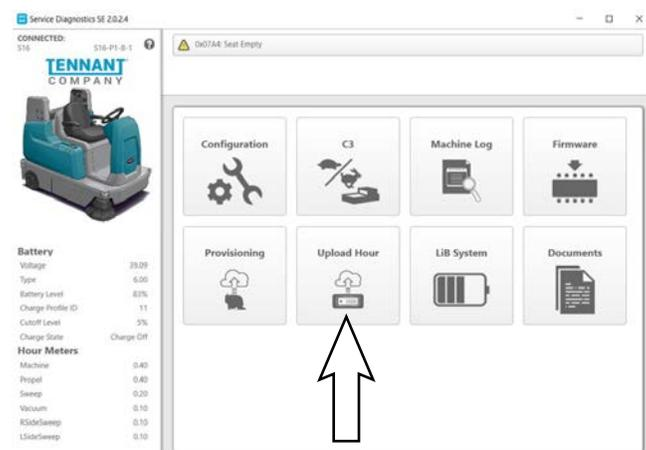
5. Click the Start Uploading Hour button to begin uploading the hour.
