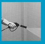
After allowing proper dwell time of disinfectant, rinse off the solution using the spray gun.
