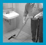
Vacuum the soil and water from the floor using the squeegee tool. The blower tool can be used to quickly dry fixtures.
