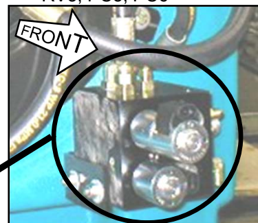
SWEEP MANIFOLD SV13, SV14, SV15, RV3, PC5, PC6
