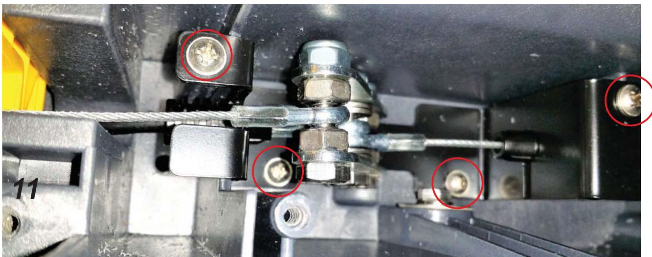
**12** Turn the splitter bracket on its side and unscrew the two screws that hold the two plastic pieces together
