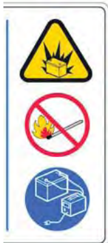
WARNING LABEL - Batteries emit hydrogen gas. Explosion or fire can result. Keep sparks and open flame away when charging. Located on bottom side of recovery tank.
