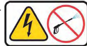
FOR SAFETY LABEL - Do not power spray or hose off machine. Electrical malfunction may occur. Located on control console
