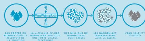
EAU PROPRE DU ROBINET DANS LE RÉSERVOIR DE LA SOLUTION LA +-CELLULE EC-H2O NANOCLEAN APPLIQUE UNE FORTE CHARGE ÉLECTRIQUE DES MILLIONS DE NANOBULLES SONT CRÉÉES LES NANOBULLES INTERAGISSENT AVEC LA SALETTE L'EAU SALE EST ÉLIMINÉE
