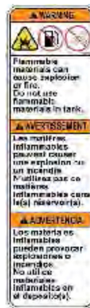
FLAMMABLE SPILLS LABEL - LOCATED ON UNDERSIDE OF SOLUTION TANK COVER.
