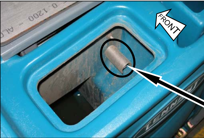
RECOVERY TANK FULL FLOAT SWITCH S4
