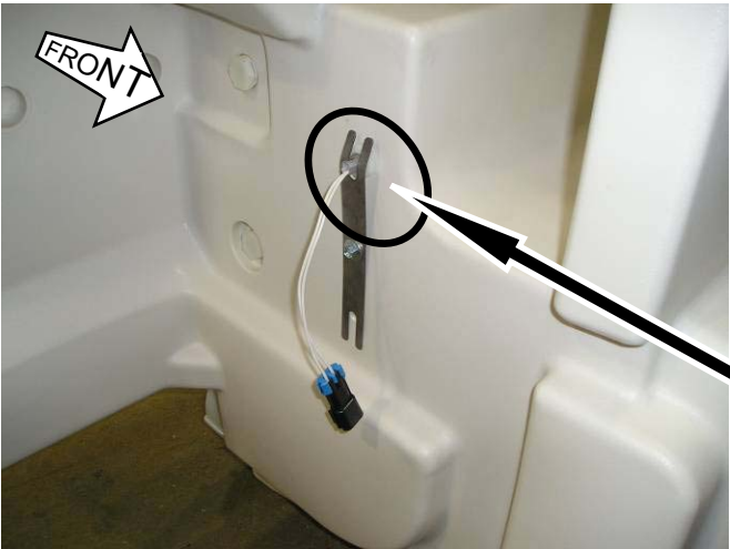
RECOVERY TANK HALF FULL FLOAT SWITCH S5
