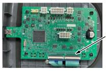
The board now has two white in- line ribbon connectors (p/n 1261320) T600 Models - Program new UI board
