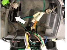
Install note: Use a small zip- tie to secure the new on/off bail switch in place.
