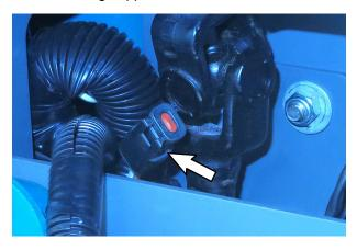
4. Disconnect resistor from main wire harness.
