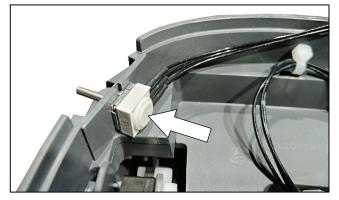
The new potentiometer is a direct replacement and does not require any specific installation instructions. To identify the difference between the previous potentiometers, the body on the new potentiometer is thinner.
