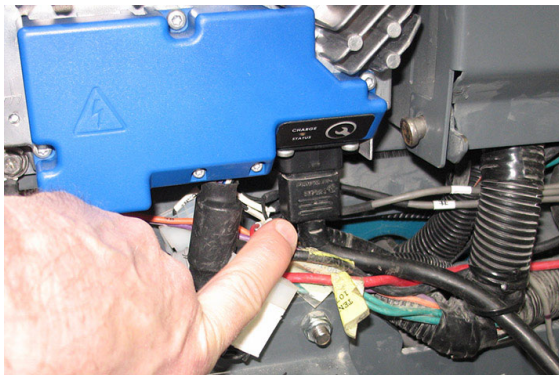
Ensure on-board charger cable is completely plugged into on-board charger.
