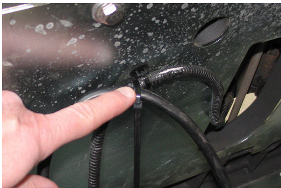
Ensure on-board charger cable is secured to seat channel and main wire harness.
