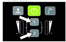
To preset the zone control buttons for different scrubbing applications, select the desired settings from list below, then press and hold the zone button until the green LED blinks three times to save preset. To preset zone 3, press and hold zone buttons 1 & 2 at the same time.
