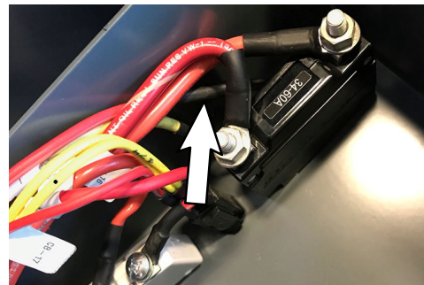
Fig. 2 - Typical Wire 150C Terminal Location
