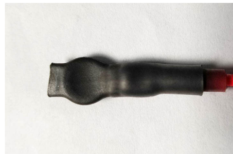
Fig. 4 - Terminal 150C Properly Covered
