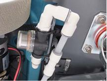
For models manufactured after the above dates, the machine frame was modified to allow the filter bowl to be orientated horizontally toward the rear of machine as shown below. This provides convenient access for filter bowl removal. A yellow maintenance touch point label was also added.
