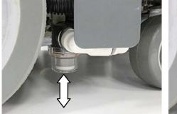
To increase ground clearance, simply rotate the filter bowl 90 degrees toward the front of the machine as shown. Re-secure with cable-ties.
