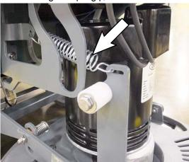
3. Using a 13mm wrench, loosen the nut on the head lift glide.
