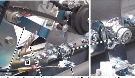
NOTE: M6 washer is required if hole diameter is 5/16" Washer (2)
