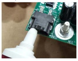
4. Fill the output connectors with the amount of grease as shown.
