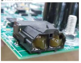
5. Reconnect wire connectors to control board.
