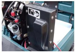
Disconnect the propel and vacuum motor wire connectors from control board as shown.
