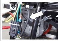
The brake wires are secured to the gearbox as shown below.
