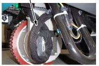
The brake wires, shown below, are routed through the harness sheathing.
