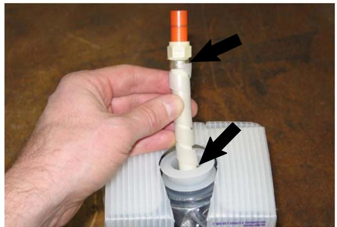
Install conduit onto FaST-PAK carton hose to prevent hose from kinking.
