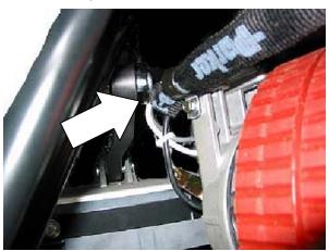
To reposition the wire harness to avoid abrasion:
