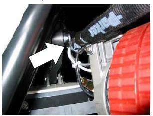
To reposition the wire harness to avoid abrasion:
