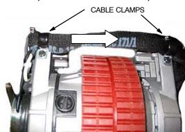
2. Secure the wires with two wire ties as shown below.
