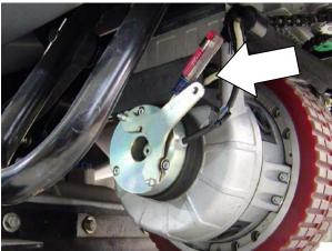
**ATTENTION:** Immediately after pushing or towing the machine, remove the screw driver from the parking brake before reconnecting the motor harness.
