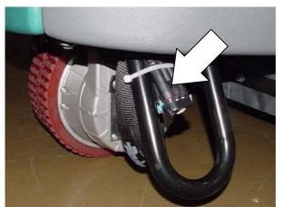
**STEP 2:** Insert a small screw driver between the electronic brake lever and hub to disable the parking brake.
