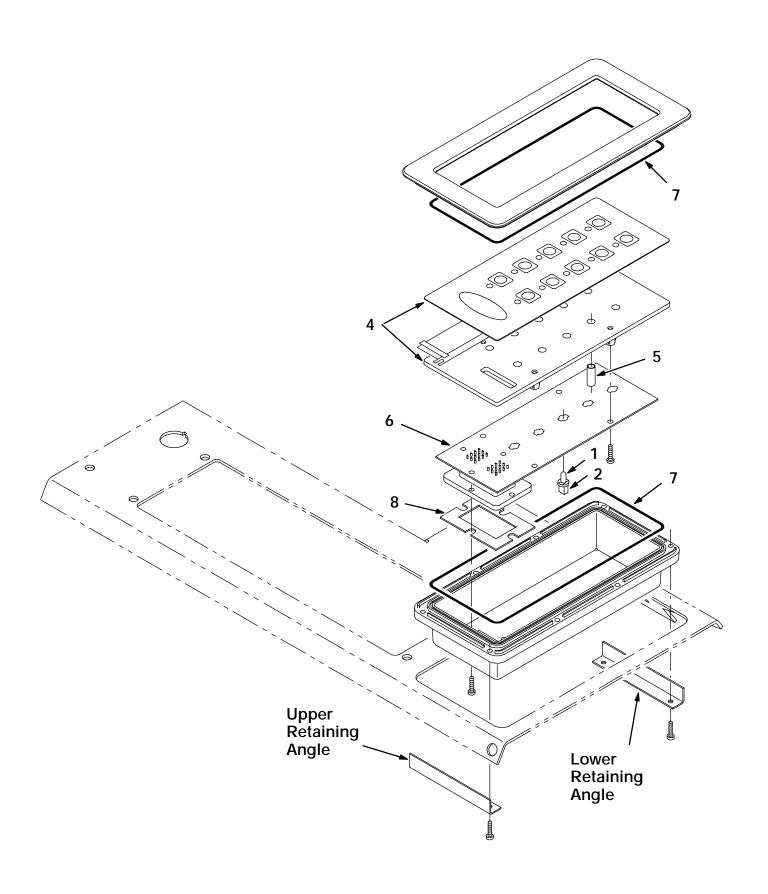
FIG. 1 – Instrument Panel Assembly
