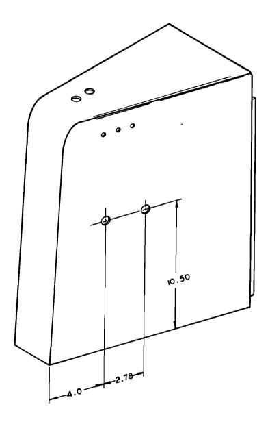
Drill two 13/32" dia. holes in the left rear corner panel as shown here. Mount the new coil strap  $^{\#}54911$ -30 and coil in this location.
