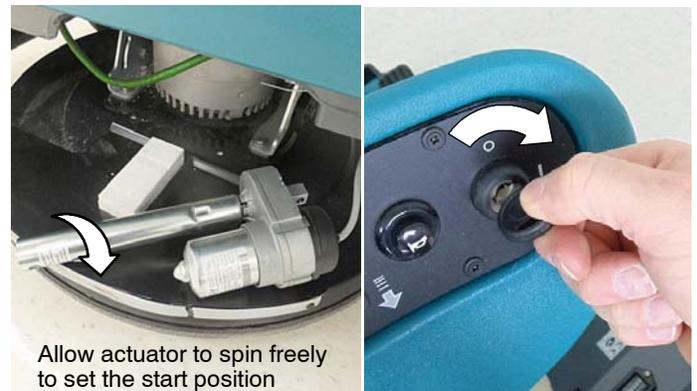
7. After the start position is set, manually turn the actuator tube until 3.25 in (8.26 cm) of thread is exposed as shown.
