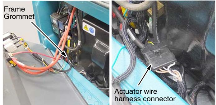
4. Carefully route the wire harness from the new actuator up through frame grommet and plug connector into the machine wire harness. **DO NOT** install actuator at this time.
