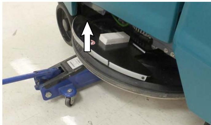
3. Remove five screws from electrical panel and lower panel to access the actuator wire harness connector. Disconnect actuator from machine harness and push connector through frame grommet. Discard defective actuator.
