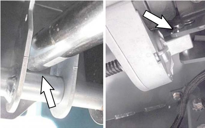
9. Center the floor jack under the burnishing head and slowly raise head until the actuator tube-end holes are aligned with mounting holes. Insert clevis pin and secure with cotter pin. Cable-tie cotter pin in place.
