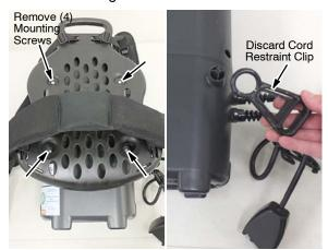
2. Using the four saved mounting screws, attach the new harness to the vacuum cleaner as shown.
