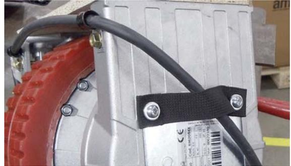
11. Connect jumper harness to the main machine harness and secure connectors to stabilizer bar with wire-ties as shown. Replace existing harness clamp with smaller clamp as shown.
