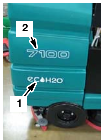
2) Label, 7100 [p/n 1047740] (Qty 2) Move the "7100" Labels to the upper position
