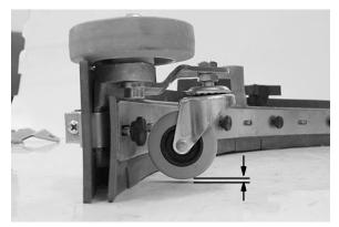
6 Attach the squeegee assembly to the machine. Lower the squeegee to floor and push the machine sightly forward. Check the blade for proper deflection. Readjust caster height if necessary.
