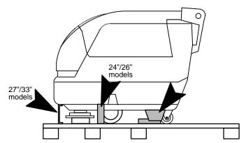
Remove the metal shipping support brackets. Make sure to reinstall nuts and washers that secure casters.
