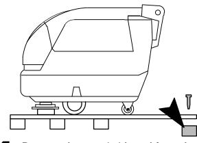
Remove the rear 4x4 board from the pallet.
