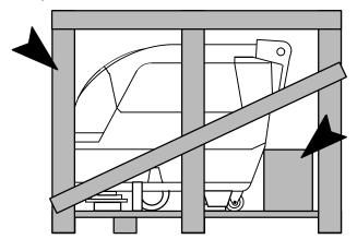
Disassemble the wooden box frame. Then remove the plastic wrap and accessories.
