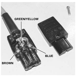
2. Reconnect wires to new plug as shown.
