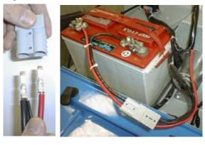
STEP 5: Disconnect wire from safety switch.
