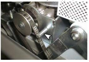
**STEP 3:** Install new belt support pin and attach belt guard with screw as shown, use a non-permanent thread lock.
