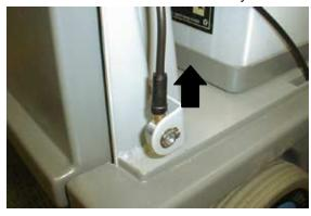
**STEP 6:** Cut off terminals and connect wires together using red butt connector. Secure wire as shown using a wire-tie provided.
