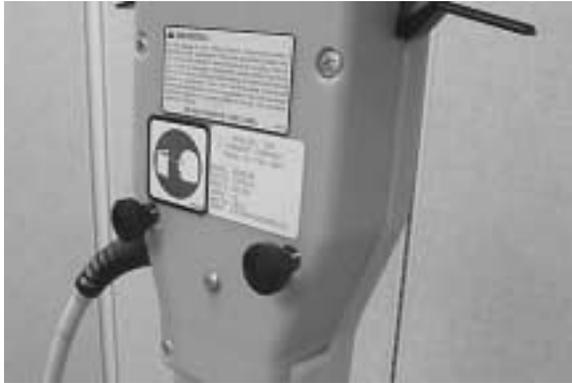
**STEP 2:** Remove existing connector bracket from spray bottle and attach new bracket from kit as shown.
