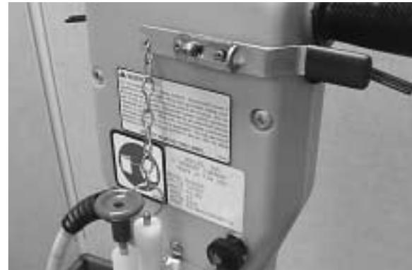
**STEP 6:** Adhere spray nozzle to machine base as shown and connect hose to bottle.
