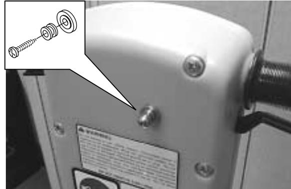
**STEP 5:** Lock trigger to latch bushing and connect chain to trigger as shown.
