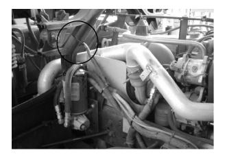
17.Lower the machine cab, and debris hopper. Check the condenser/drier for proper operation.
