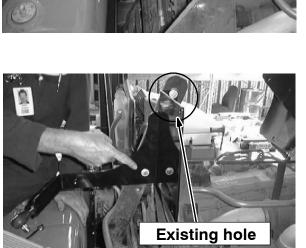
8. Secure bracket 1012834 to the existing angle where the flat plate was removed in step 4, using M8 screw 09011, 5/16 washer 32491 and M8 nut 08709. This will help stabilize the condenser.
