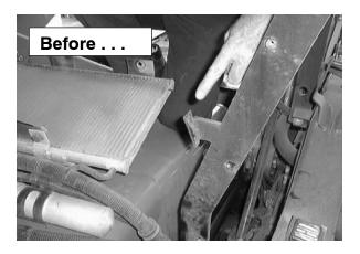
. . and remove the existing ear with a cutting wheel.
