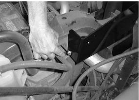
12. Reposition the drier, and clamp it to the bracket, using the hole behind the mounting point, clamp 41016, M8 screw 09740, 5/16 washer 32491 and M8 flange nut.
