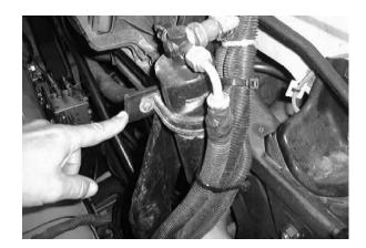
2. ,After removing all condenser and drier mounting hardware, lay the condenser and drier back on the fuel tank.
