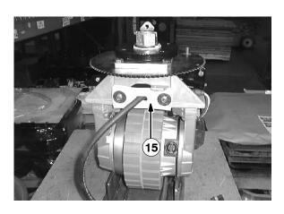
15.Install brake arm (2) with hex screw (3) and lock nut (4).
