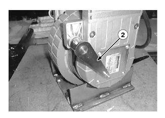
16. Install brake link (15) to brake brake arm (2) with cotter pin 39005. Mount the brake arm (2) in the third hole of the brake link (15) as shown.
