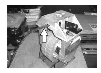
13.Install caster bearing and brake link 81685. Connect brake link 81685 to brake lift arms with clevis pin 36191 and cotter pin 08170.
