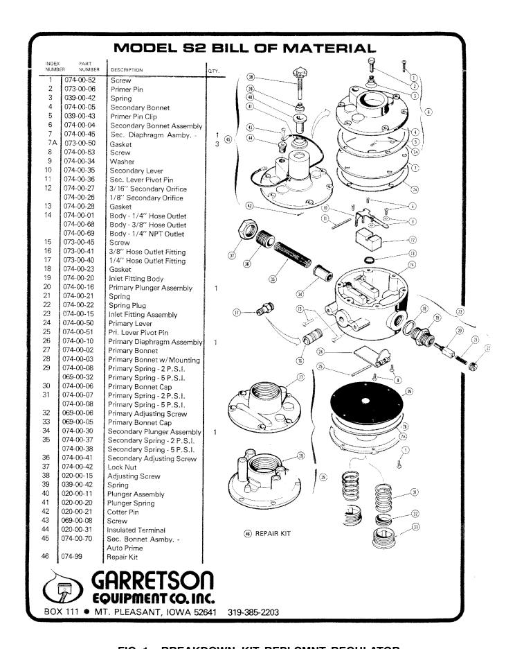
FIG. 1 - BREAKDOWN, KIT, REPLCMNT, REGULATOR
