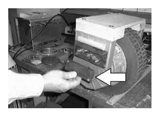
4. Remove the two screws holding the electrical box.
