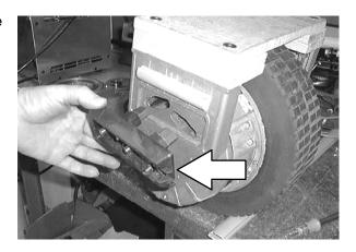
6. Remove the screws and nuts holding the brushes in place.
