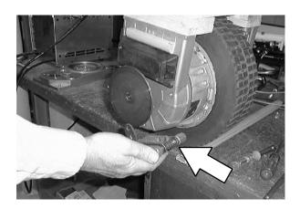
2. Remove the rotor from the front drive wheel and set aside.
