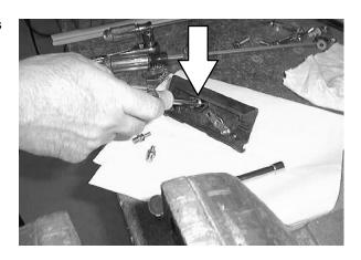
7. Remove and discard the old motor brushes. Set the mounting hardware aside.
