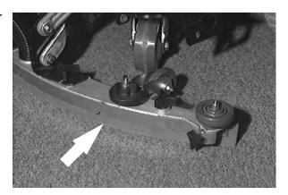
5. If the deflection is not the same over the full length of the blade, turn the squeegee leveling knob counter-clockwise to increase the deflection at the ends of the squeegee.
