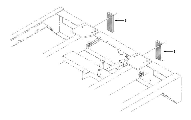
FIG. 2 - RUBBER BUMBER INSTALLATION
