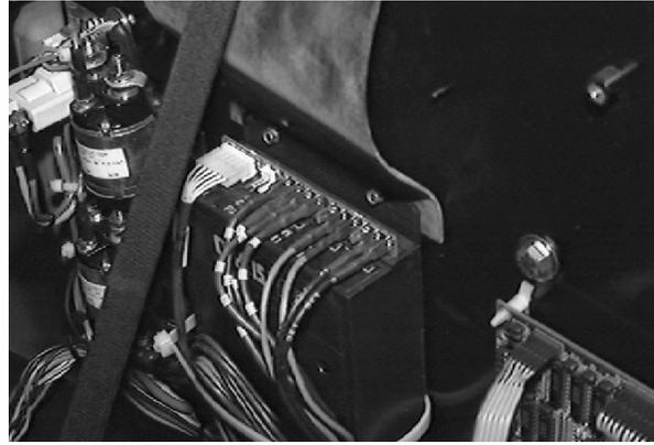
5. Unplug the potentiometer from the controller. Unplug the wire harness from the stop switch and the ribbon cable from the controller. Remove and set aside the speed control handle latch. Remove the shroud locking bracket from behind the shroud. Slide the adjustable steering housing out of the slots in the fixed steering housing. (Refer to FIG. 1)
