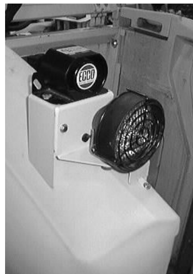
FIG. 8 - Backup alarm assembly installation
