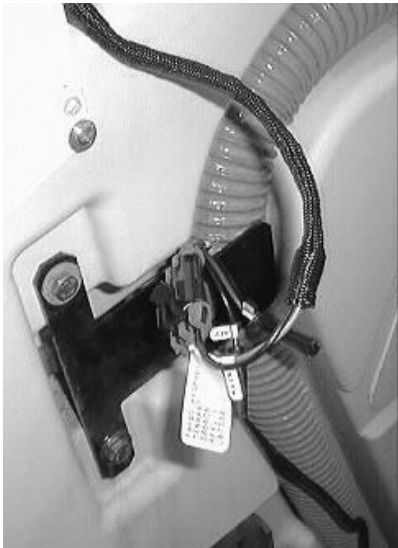
FIG. 9 - Connect backup alarm to main wire harness
