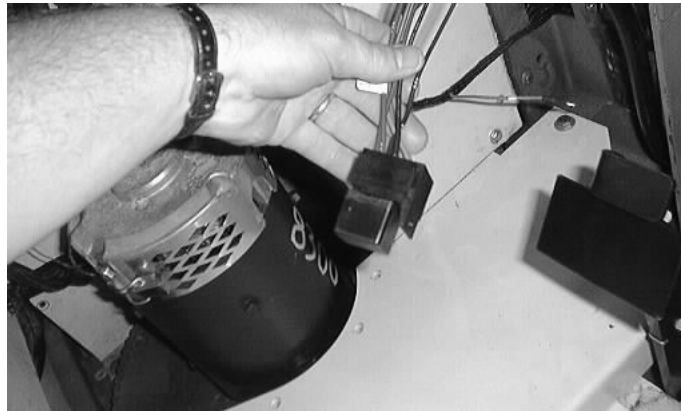
FIG. 6 - Mount relay to main wire harness
