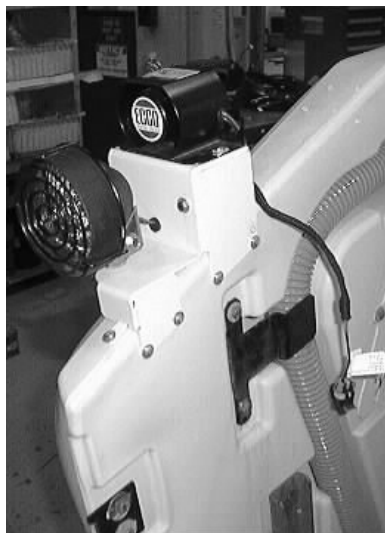
FIG. 7 - Backup alarm assembly installation
