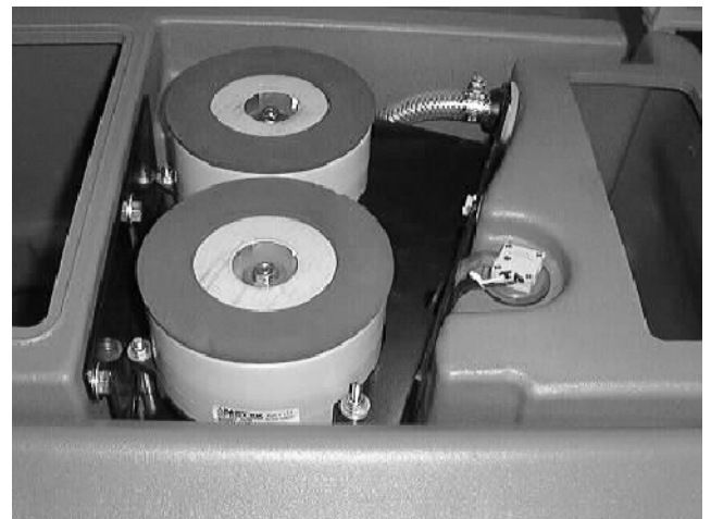
FIG. 5 -Dual Vacuum Fan Assembly Installation
