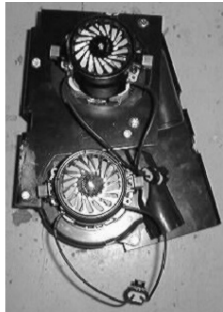
FIG. 3 - Dual Vacuum Fan Assembly (Top And Bottom View)
