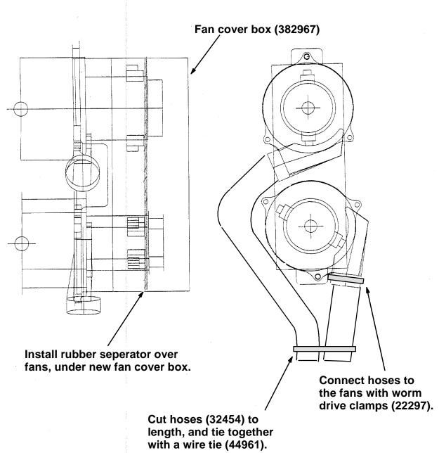
FIG. 2 - NEW FAN COVER BOX ASSEMBLY
