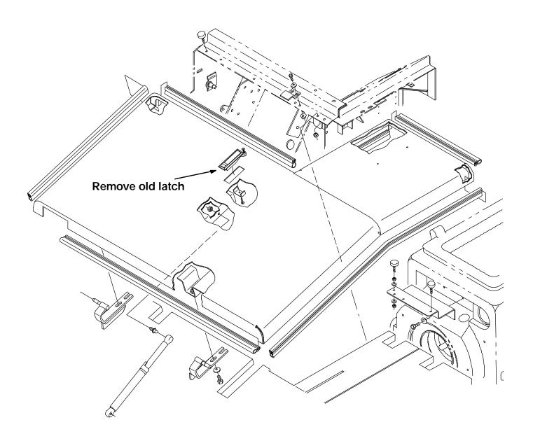
FIG. 1 - Engine Cover Latch Removal
