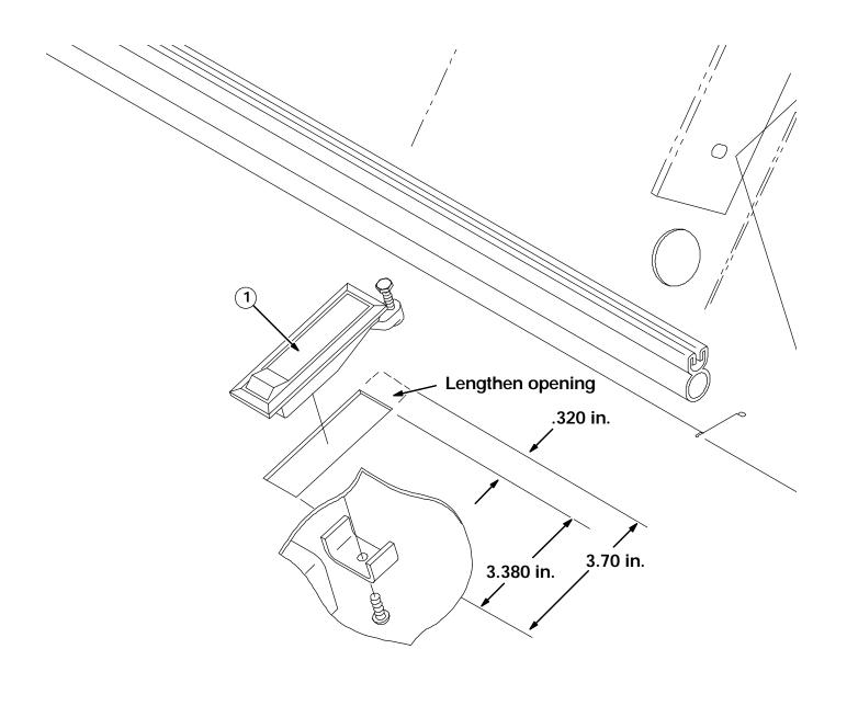
FIG. 2 - REPLACEMENT LATCH INSTALLATION
