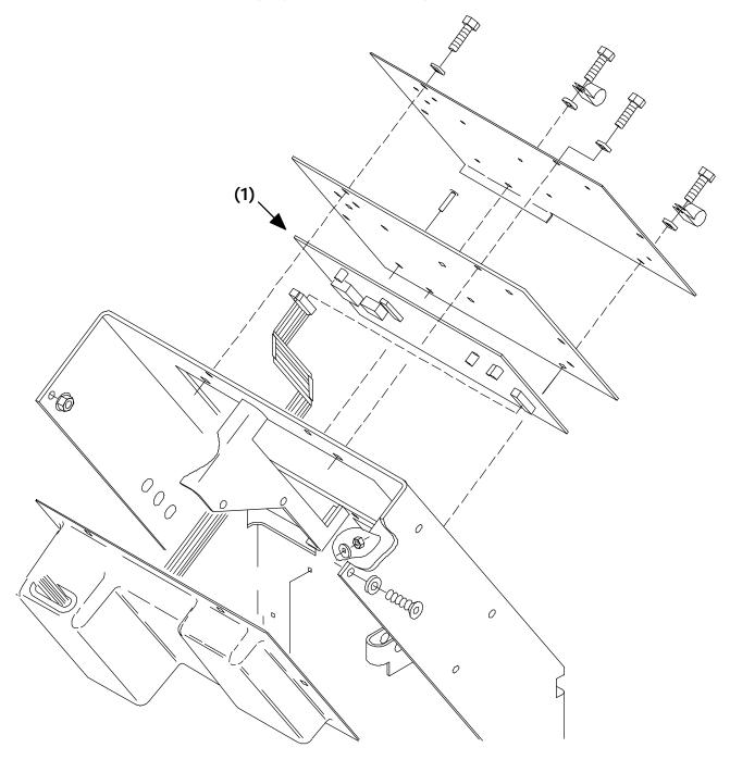
FIG. 1 - Controller Assembly
