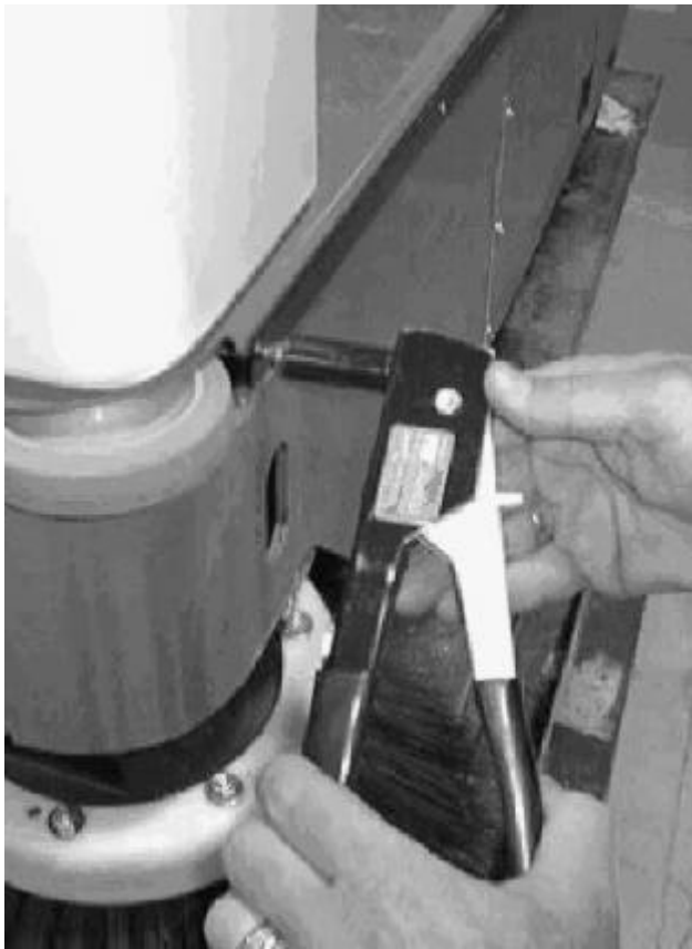
FIG. 4 - MOUNT RETAINER WITH RIVETS AND SLIDE ON BUMPER STRIPS
