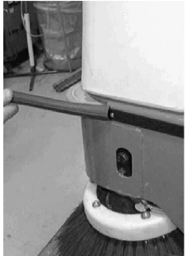
FIG. 4 - MOUNT RETAINER WITH RIVETS AND SLIDE ON BUMPER STRIPS
