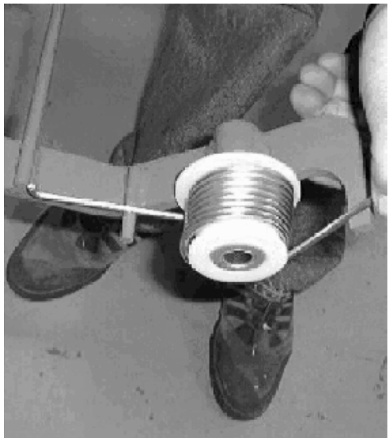
FIG. 9 - MOP FRAME WELDMENT SPRING INSTALLATION
